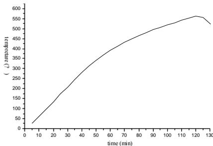
Fig. 6 Stirrup temperature distribution versus time curve
