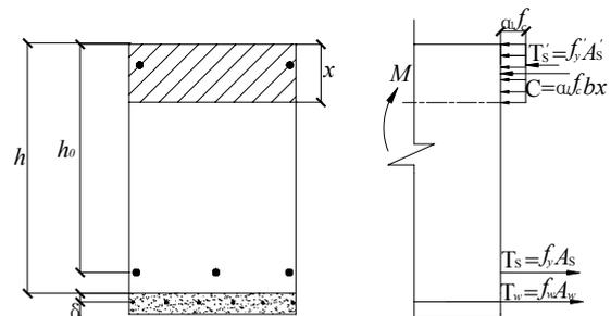
Fig.7 Calculating graph of flexural capacity
