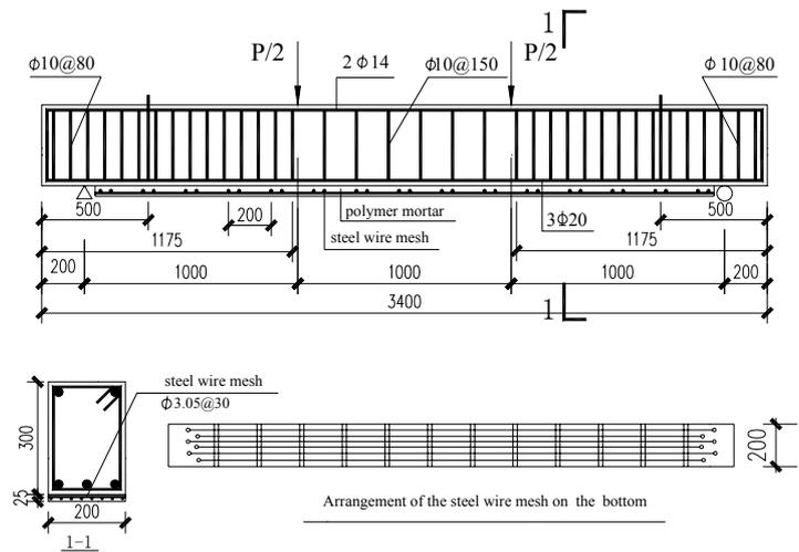
Fig. 2 Arrangement of the steel wire mesh
