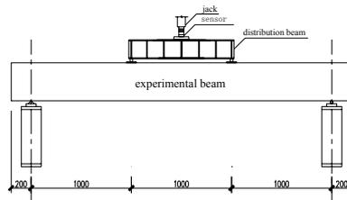
Fig. 3 Test setup
