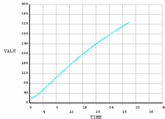
Fig. 5 Steel temperature curves at mid span
