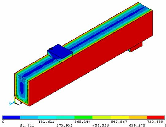
Fig. 4 Distribution of temperature after 30 min
