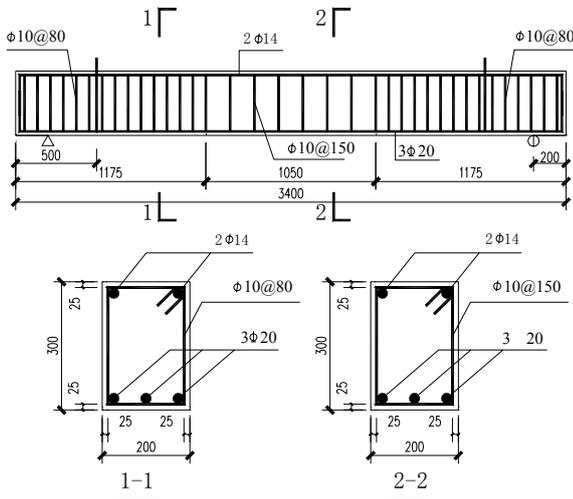
Fig. 1 Dimensions of specimens and arrangement of reinforcement
