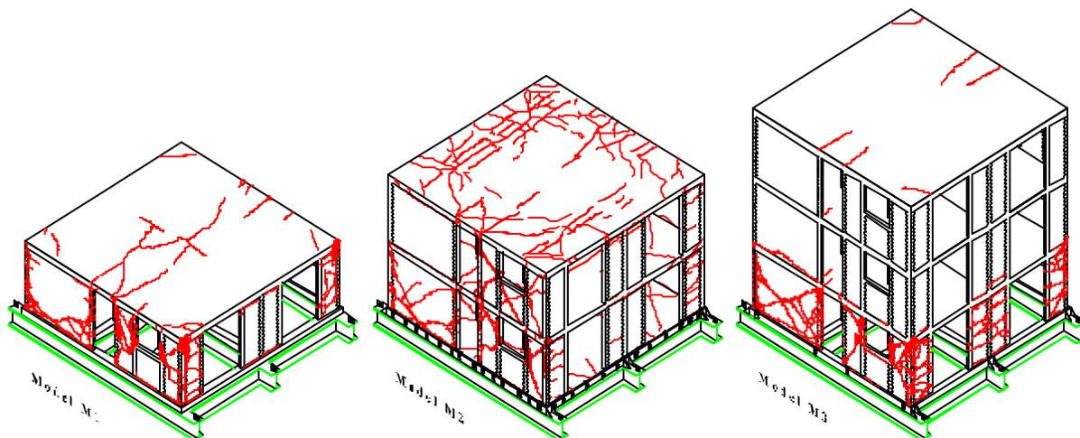
Figure 2. Final cracks patterns
