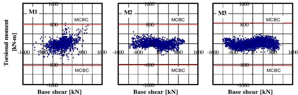
Figure 8. Torsional moment and base shear hysteretic loops for maximum limit state
