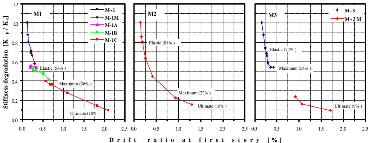
Figure 5. Stiffness degradation
