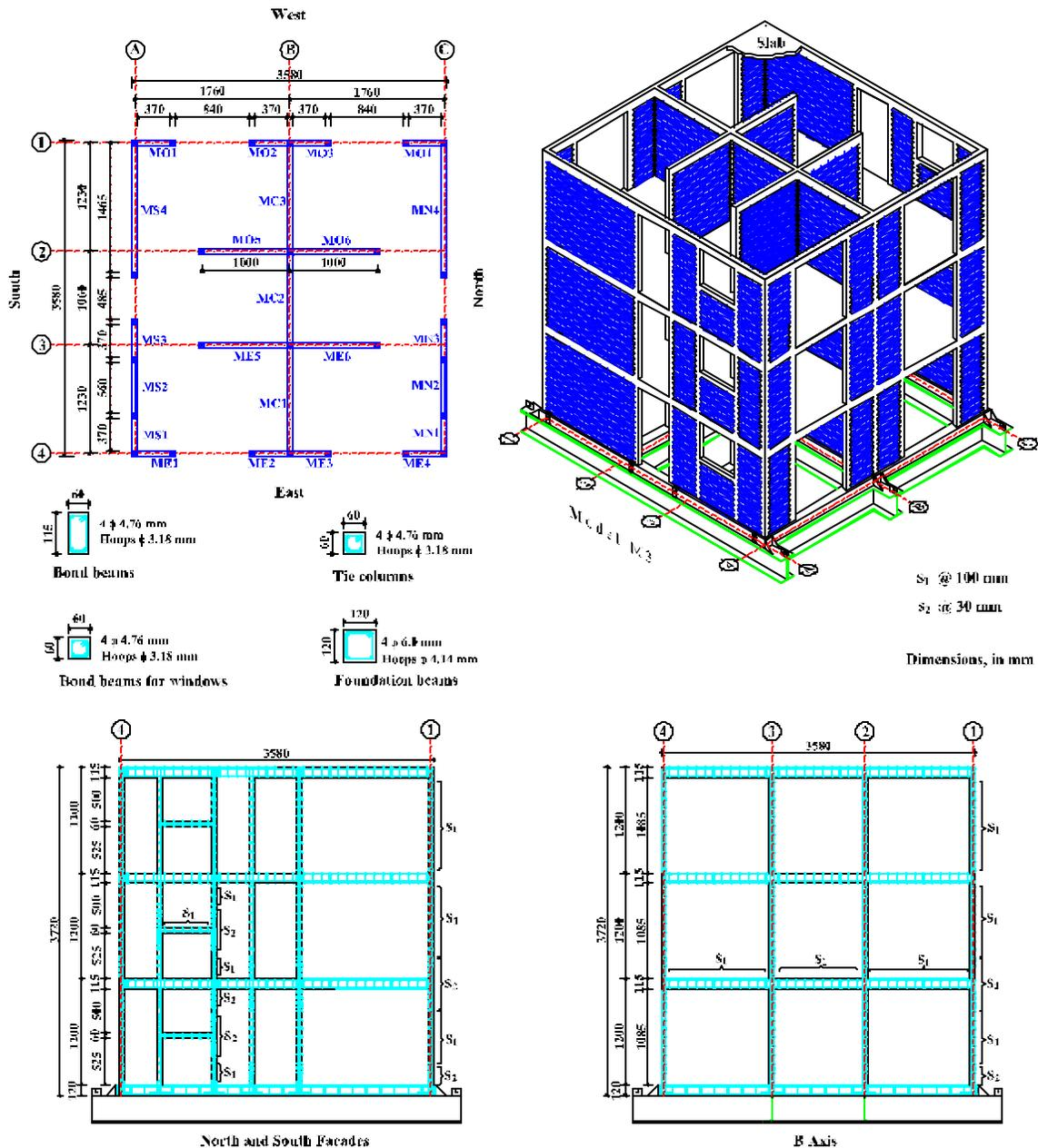
Figure 1. Characteristics of the specimens
