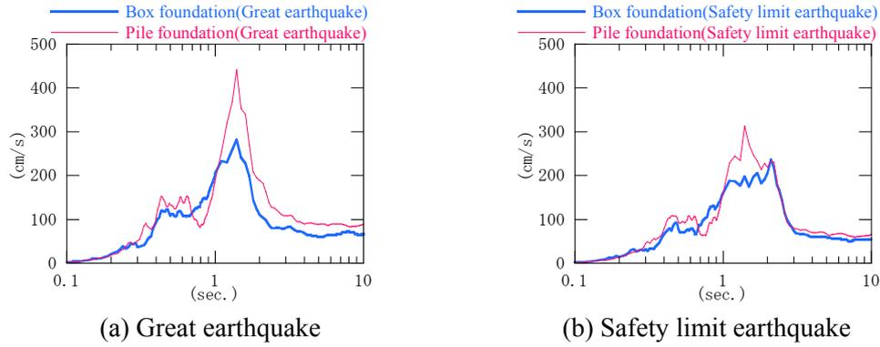
Figure 8 Comparison between response spectrum of box foundation and that of pile foundation
