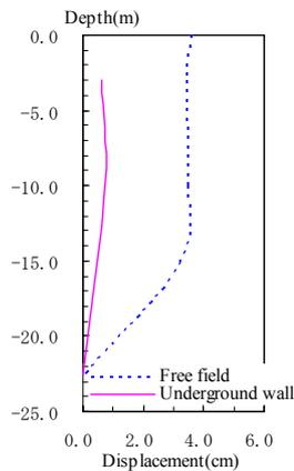
Figure 5 Displacement distribution of free field and continuous underground wall
