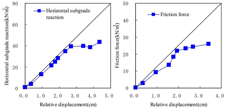
(a) Horizontal subgrade reaction (b) Friction force
