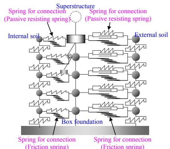
Figure 9 Outline of passive resisting springs and friction springs    Figure 10 Proposal dynamic analysis model
