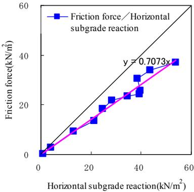
Figure 3 Relation between friction force and horizontal subgrade reaction of continuous underground wall
