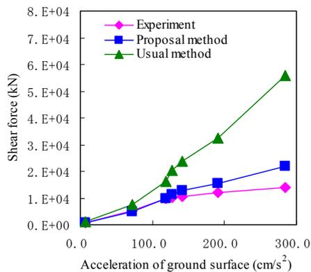
Figure 12 Analysis results on shear force of continuous underground wall
