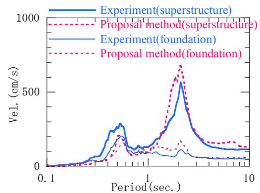
Figure 15 Comparison of response spectra between the proposal method results and the experiment results
