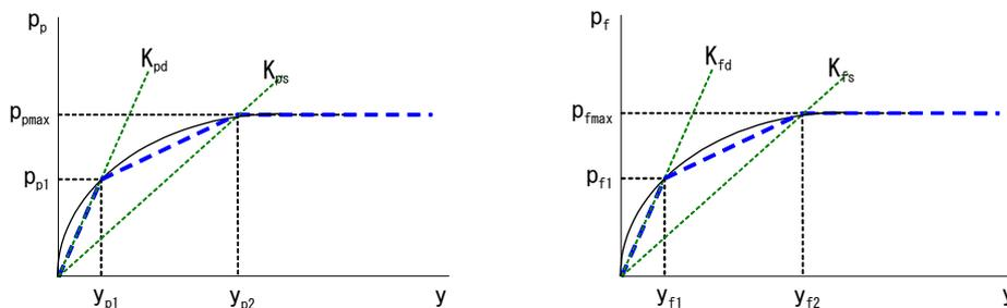
(a) Horizontal subgrade reaction – displacement    (b) Friction force - displacement
