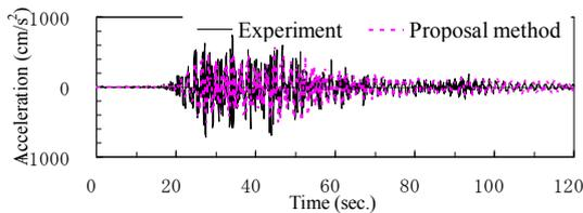
Figure 14 Comparison of waves between the proposal method result and the experiment result
