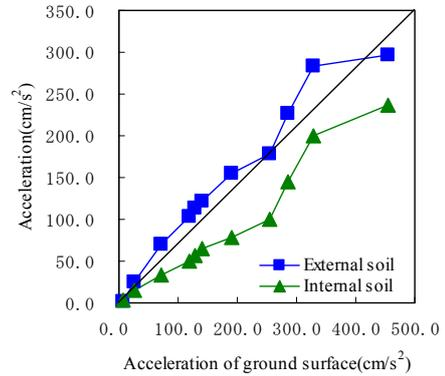
Figure 6 Comparison between acceleration of internal soil and that of external soil
