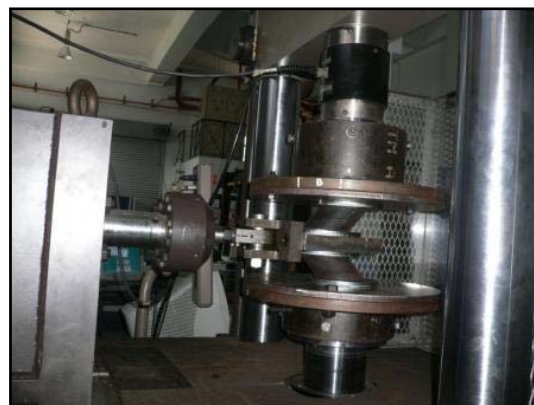
Figure 11 Cyclic test loading of rubber bearing
