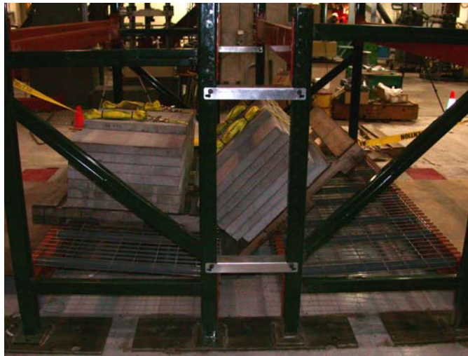
Figure 6: Pallets at the end of test with a motion from the amplified reduced ATC-63 set – Test P9_121211, after Sideris (2008)
