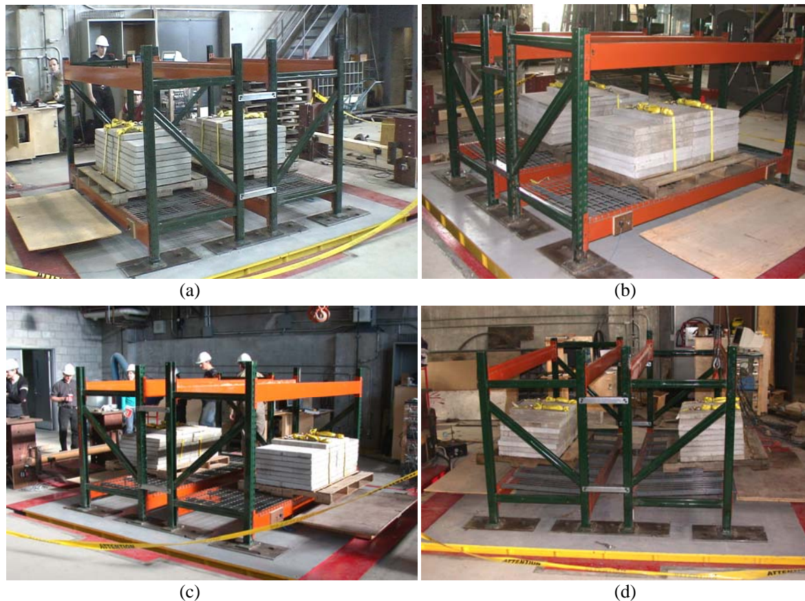
Figure 3: Specimen configurations: (a) Centered pallet and horizontal shelf, (b) Centered pallet and inclined shelf, (c) Eccentrically placed pallet and horizontal shelf, (d) Eccentrically placed pallet and inclined shelf
