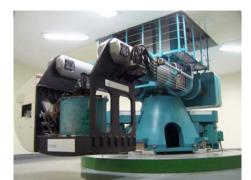
(a) The full view of the facility under construction (b) The installed centrifuge Figure 4 Geotechnical centrifuge facility
