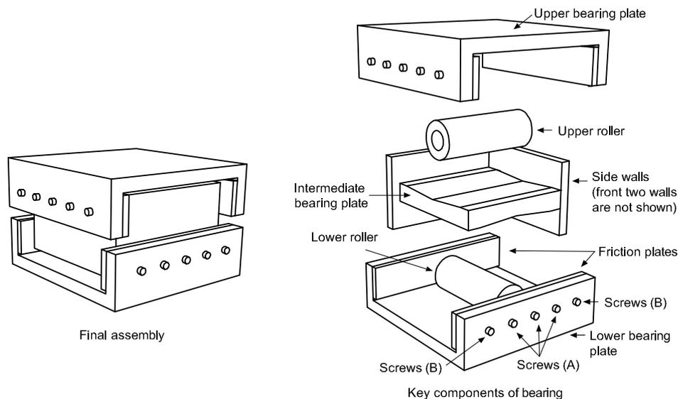
Figure 1 Simplified schematic view of roller seismic isolation bearing
