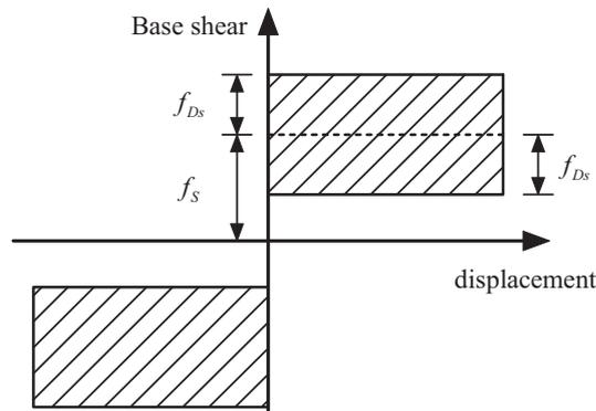
Figure 4 Base shear versus horizontal displacements
