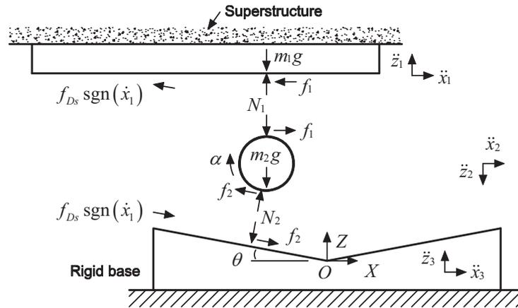
Figure 2 Free body diagram when the roller is on the left
