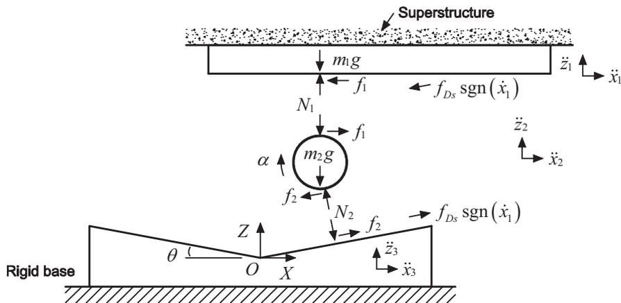
Figure 3 Free body diagram when the roller is on the right
