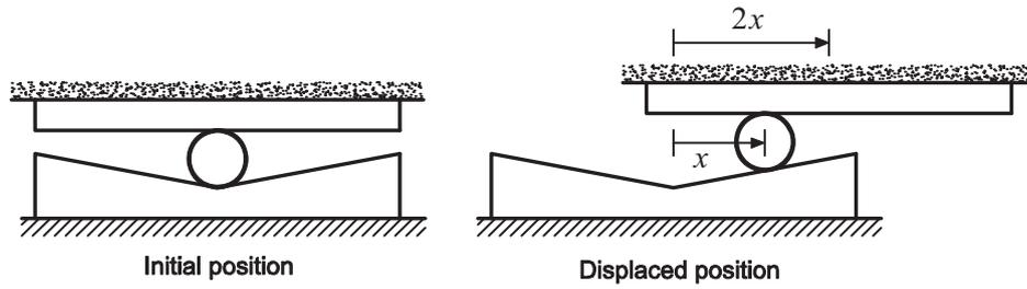
Figure 5 Relationship between displacements of the roller and superstructure
