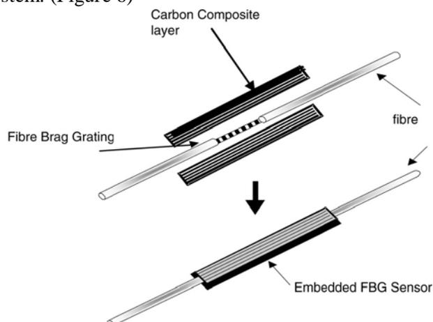
Figure 5. Strain Sensor Placed Between Layers of Composite Material.
