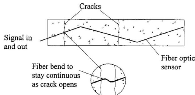
Figure 9. Principle of Operation of the Zigzag Sensor
