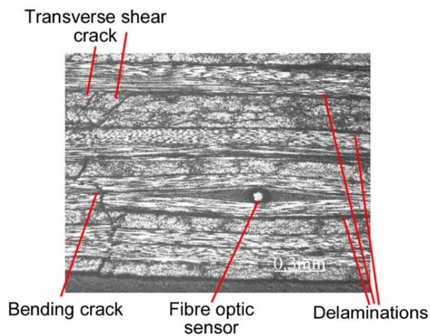
Figure 12. Section through Damaged Area of FRP Containing Fiber Optic
