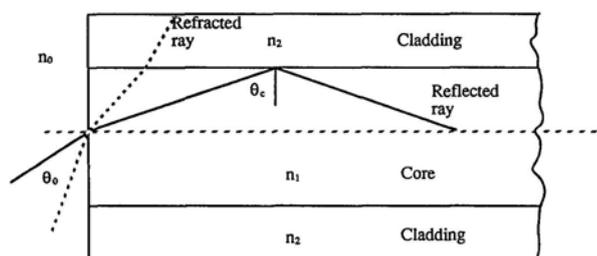
Figure 2. Basic Geometry of Optical Fiber Sensor
