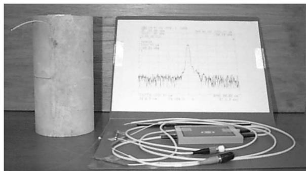
Fig. 15. A Concrete Cylinder with an Embedment of FBG Sensor (left)
