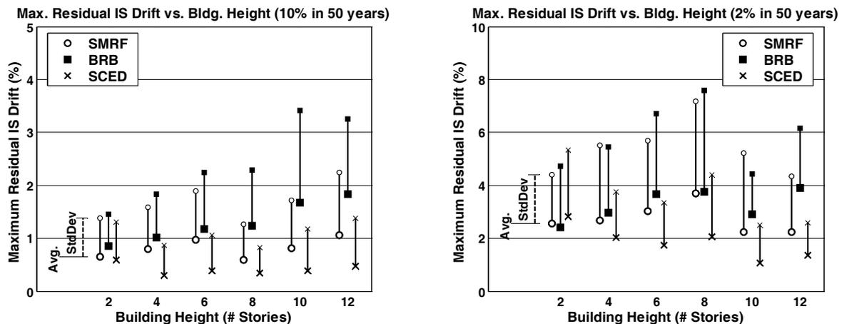
Figure 5 Mean Maximum Residual Interstory Drift vs Building Height and Type
