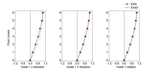
Figure 4. Mode shapes extracted from reconstructed responses using proposed modal identification method
