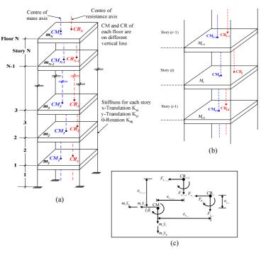
Figure 1. Torsionally coupled multi-storey building
