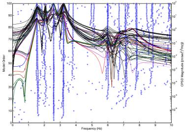
Figure 3. Frequency stability diagram superimposed with the CPSD functions
