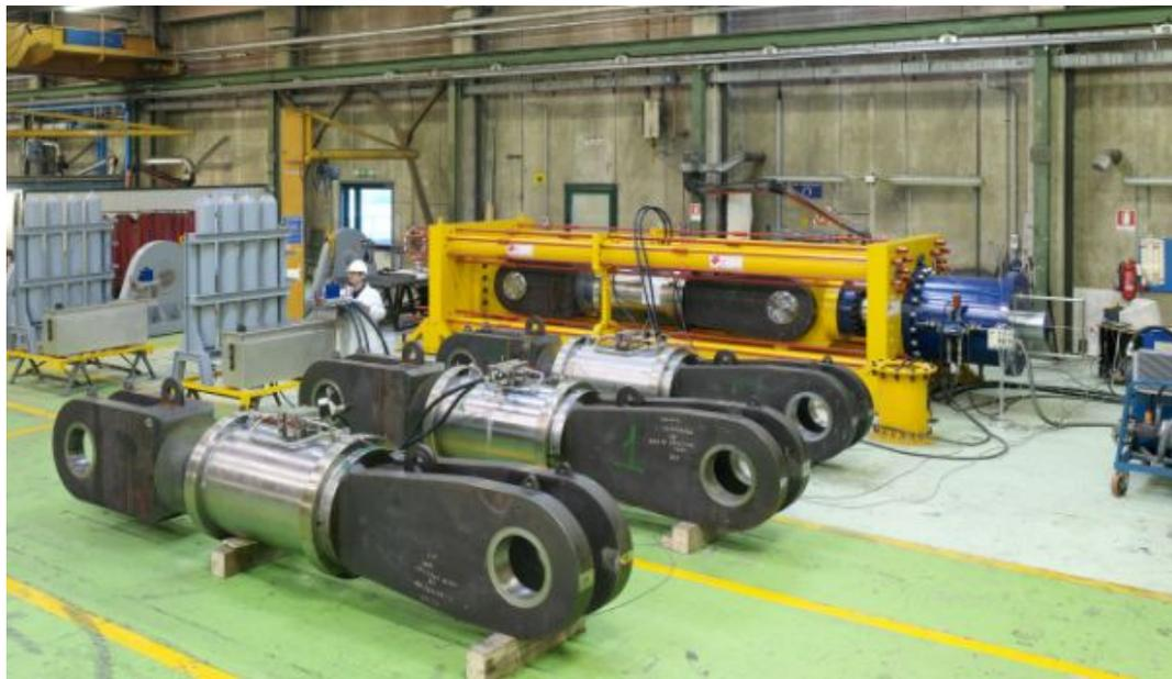
Figure 4. STUs under testing at FIP Industriale Laboratory.
