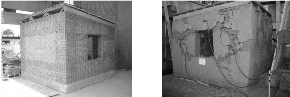
Figure 10 Adobe model reinforced with plastic mesh
