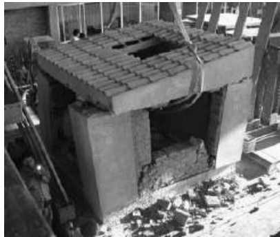
Reinforced model after seismic test
