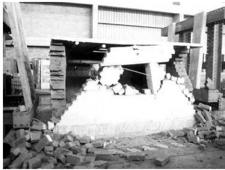
Figure 6 Adobe models after seismic tests. L: Unreinforced. R: Reinforced with cane
