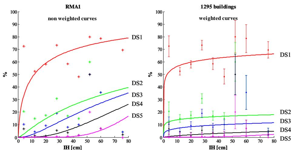
Figure 4 Comparison of non weighted and weighted fragility curves in  $I_H$  for RMA1.
