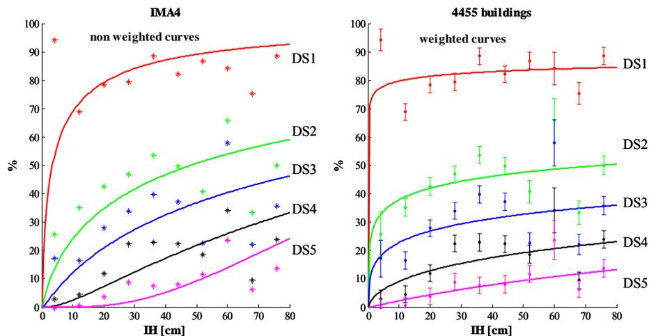
Figure 3 Comparison of non weighted and weighted fragility curves in  $I_H$  for IMA4.
