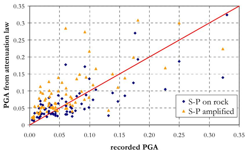
Figure 1 Comparison of recorded PGA and PGA evaluated with the Sabetta and Pugliese (S-P) [1987] attenuation law, on rock (blue diamonds) and amplified to account for site effects (orange triangles).
