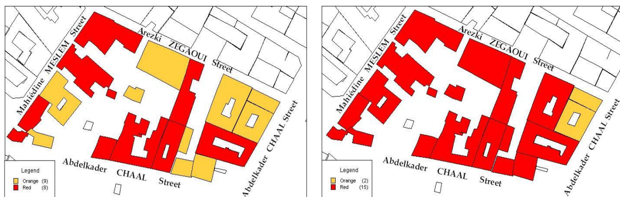
Figures 3 and 4 Classification of the area 135 buildings before and after the Zemmouri earthquake
