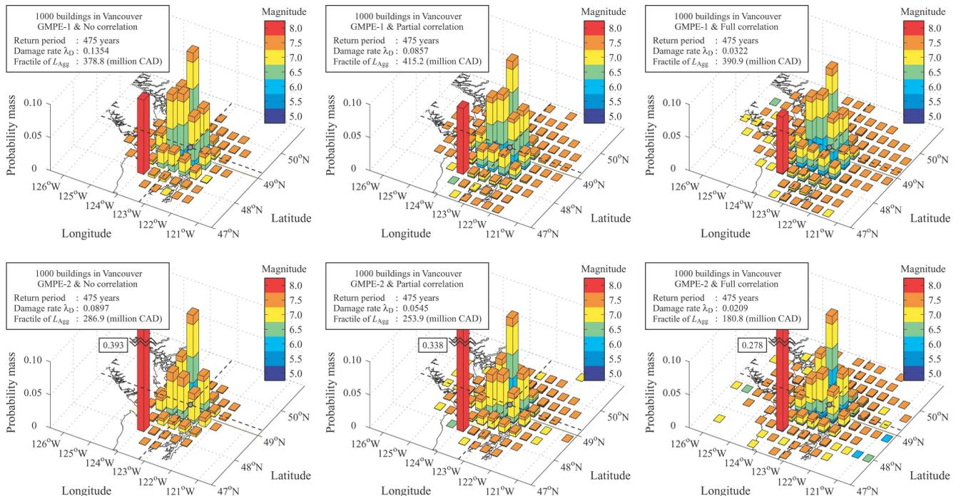
Figure 4 Geographic deaggregation of  $L_{Agg}$  of 1000 buildings for the 475-years return period considering three correlation cases and using GMPE-1 (top) and GMPE-2 (bottom)
