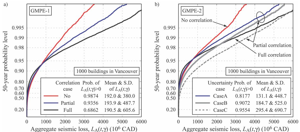
Figure 2 Probability distributions of  $L_A(t, \gamma)$  of 1000 buildings plotted on Gumbel probability paper considering three correlation cases: a) GMPE-1 and b) GMPE-2
