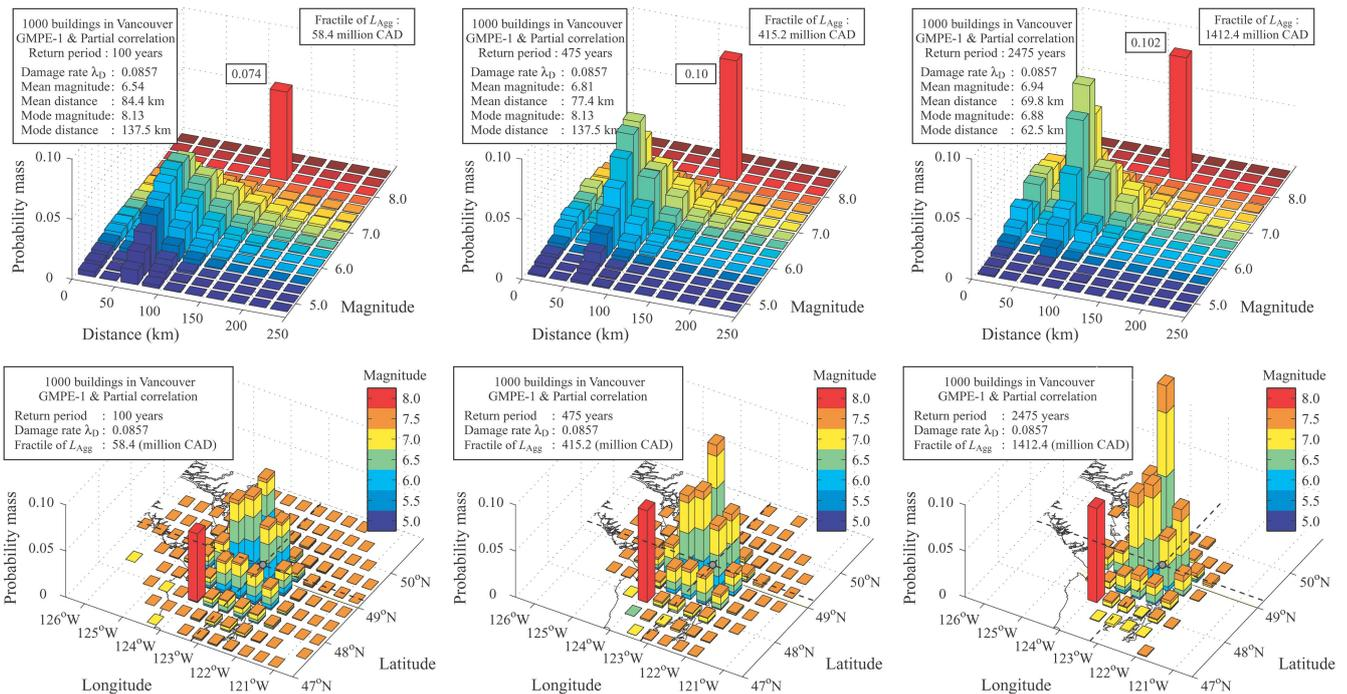
Figure 5 Deaggregation of  $L_{Agg}$  of 1000 buildings for the return periods of 100, 475, and 2475 years considering the partial correlation case and using GMPE-1
