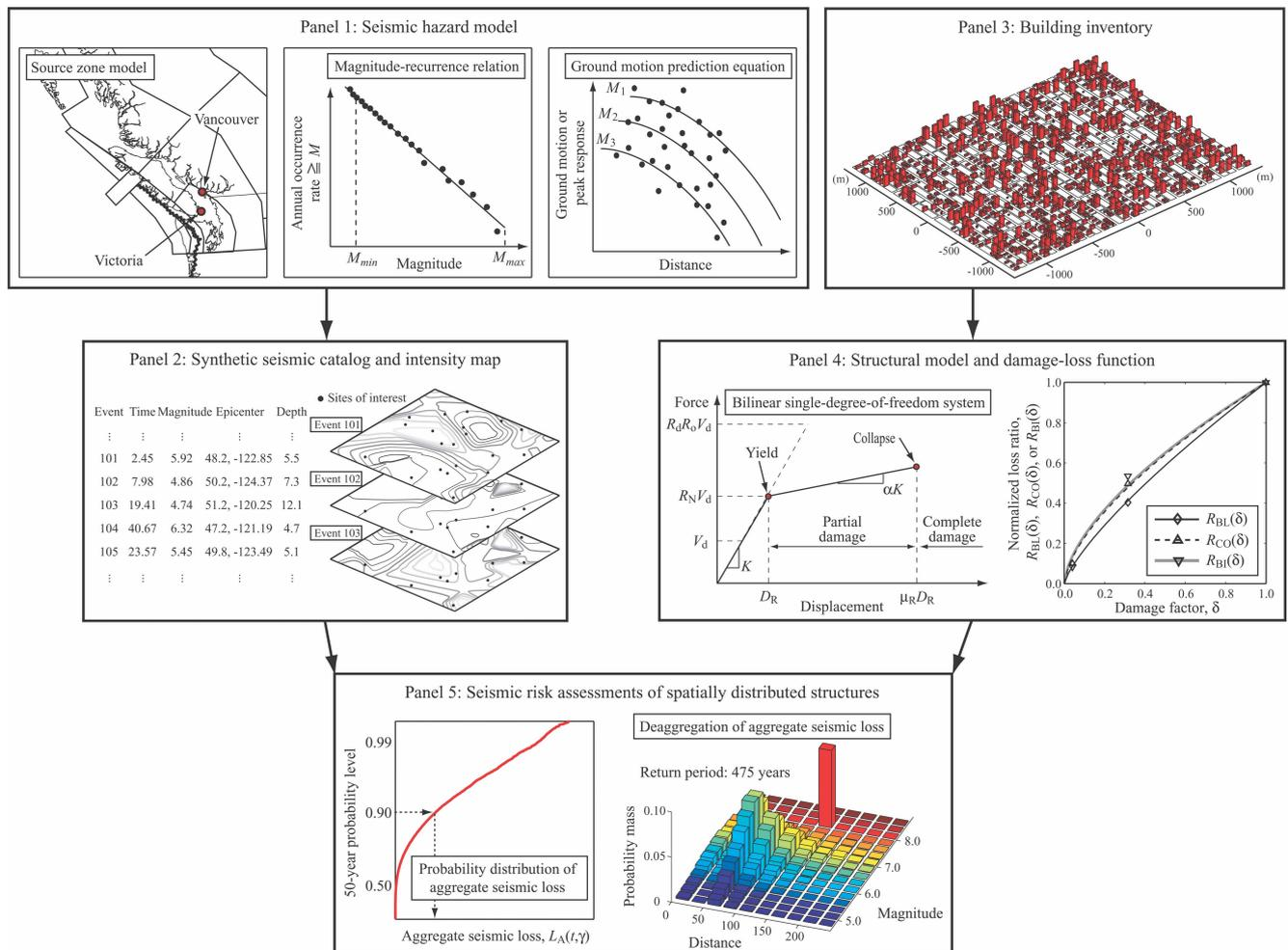
Figure 1 Seismic risk assessment procedure for spatially distributed structures: Panel 1) seismic hazard model, Panel 2) seismic catalog and intensity map, Panel 3) building inventory, Panel 4) structural model and damage-loss function, and Panel 5) seismic risk assessment of spatially distributed structures
