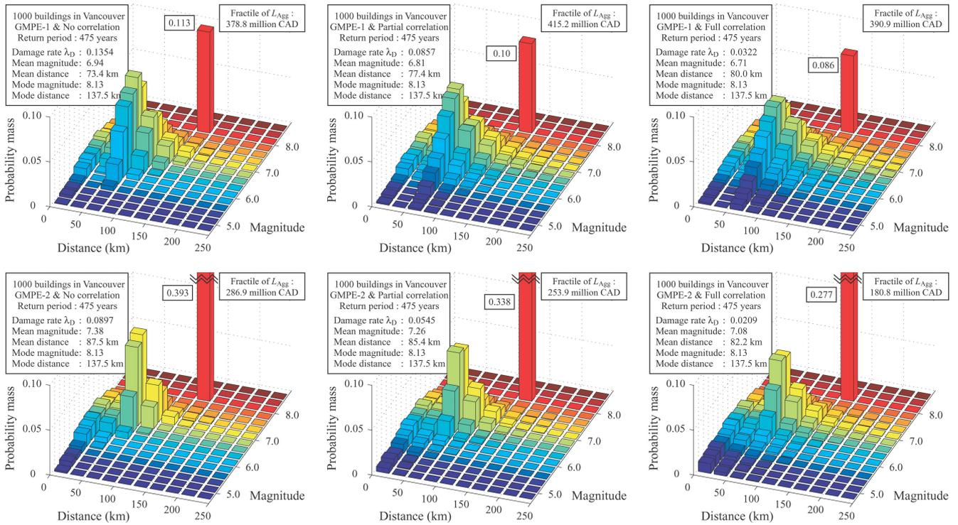
Figure 3 Deaggregation of  $L_{Agg}$  of 1000 buildings for the 475-years return period considering three correlation cases and using GMPE-1 (top) and GMPE-2 (bottom)
