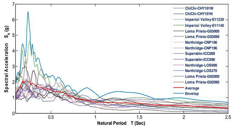
Fig. 2 Scaled ground motion spectra
