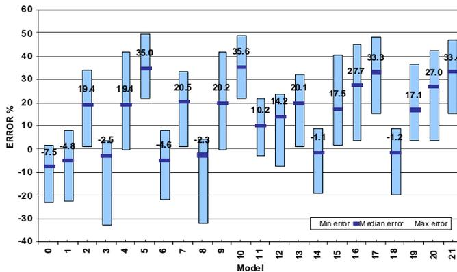
Fig. 7 Relative errors of estimated frame base shears
