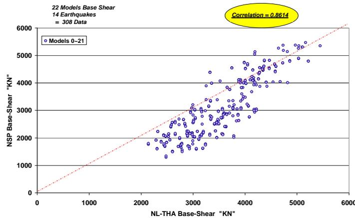
Fig. 6 Scatter plot of estimated frame base shears
