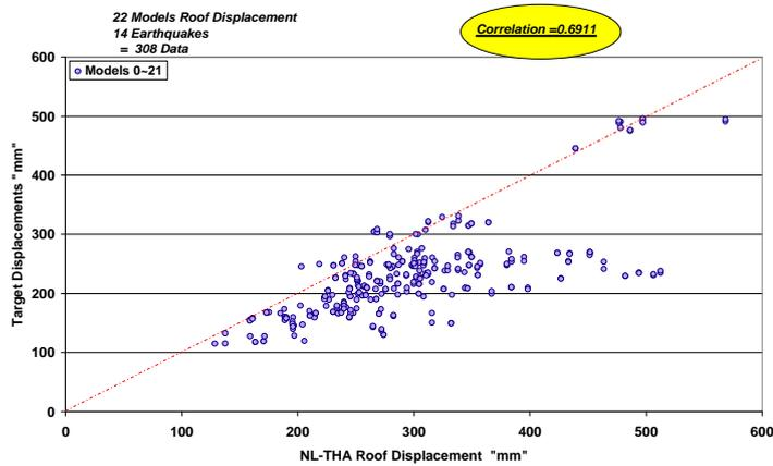
Fig. 4 Scatter plot of estimated maximum roof displacements
