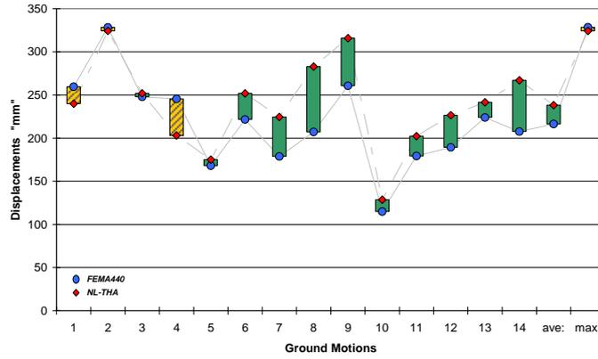
Fig. 3 Estimated maximum roof displacements for frame model 0
