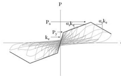
Figure 2.2: Bounding Backbone Curve Used for Model Calibration
