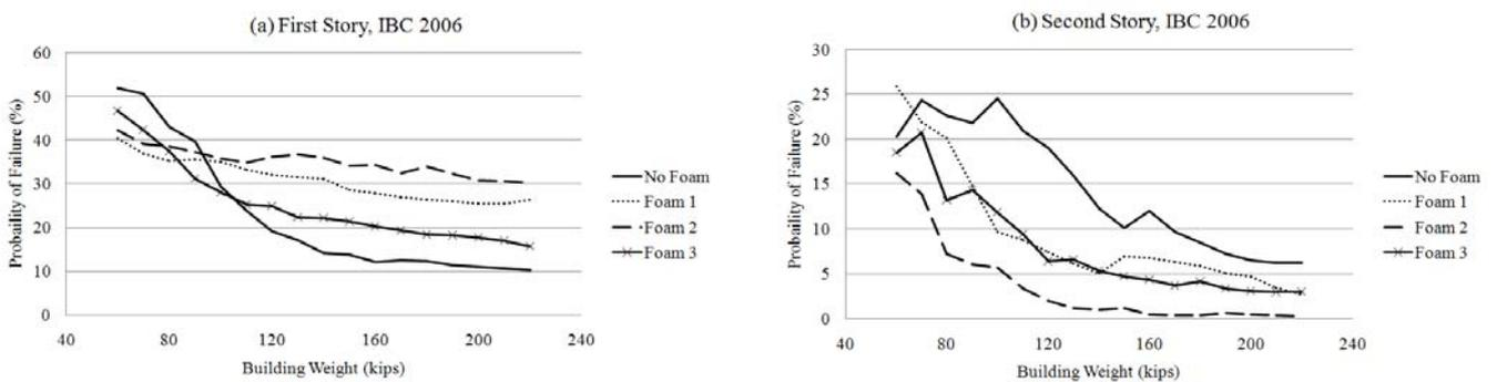
Figure 3.7: Two-Story Probability of Failure Results for Design Level Earthquake Using IBC 2006
