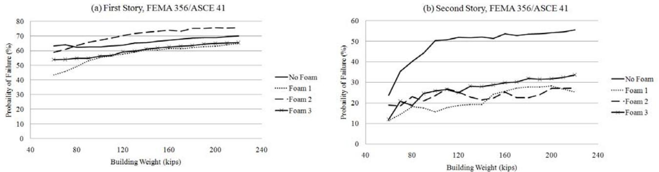
Figure 3.6: Two-Story Probability of Failure Results for Design Level Earthquake Using FEMA 356/ASCE 41
