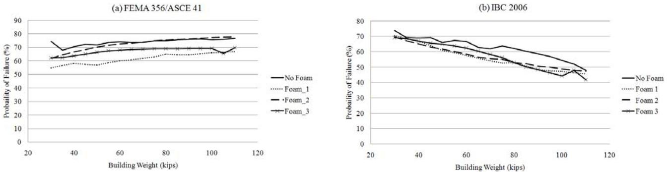
Figure 3.5: One-Story Probability of Failure Results for Design Level Earthquake for FEMA 356/ASCE 41(a) and IBC 2006(b)
