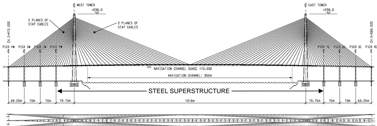
Figure 1 Elevation and plan
