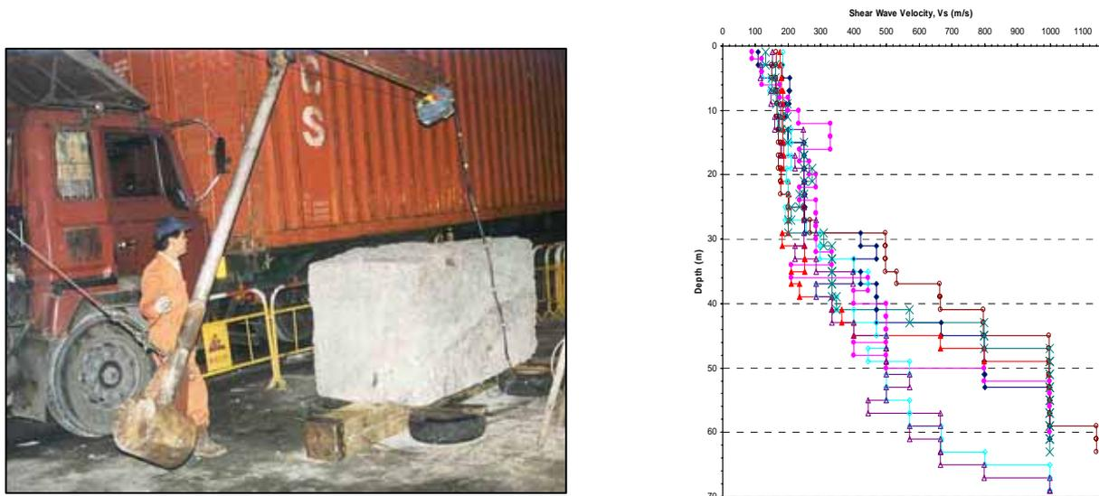
Figure 4 Insitu shear wave testing and derived  $G_0$  profiles
