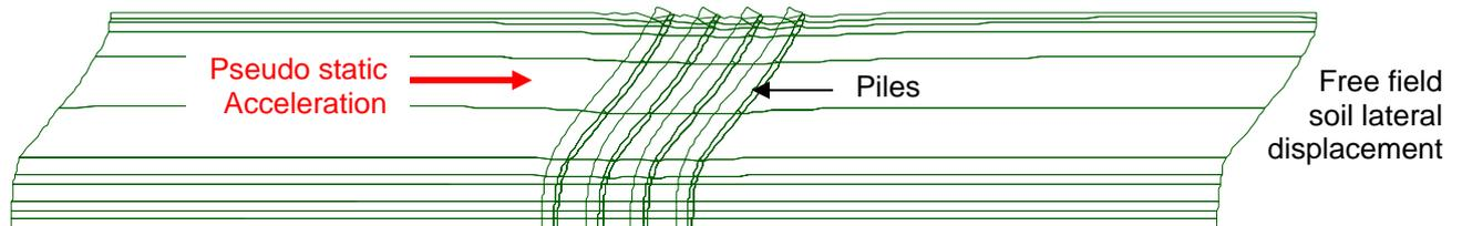
Figure 8 Pile movements below the soil surface
