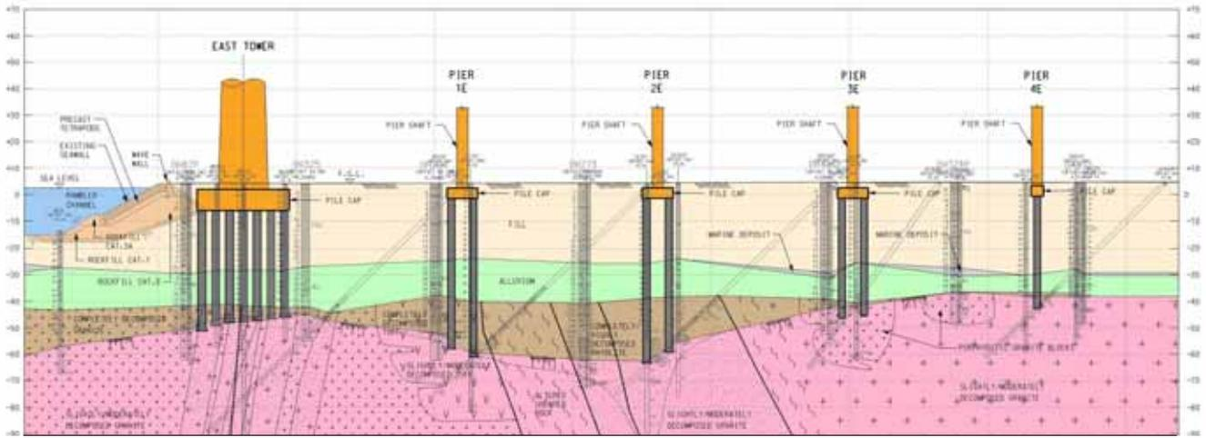
Figure 7 Section through the East Tower and Back Spans
