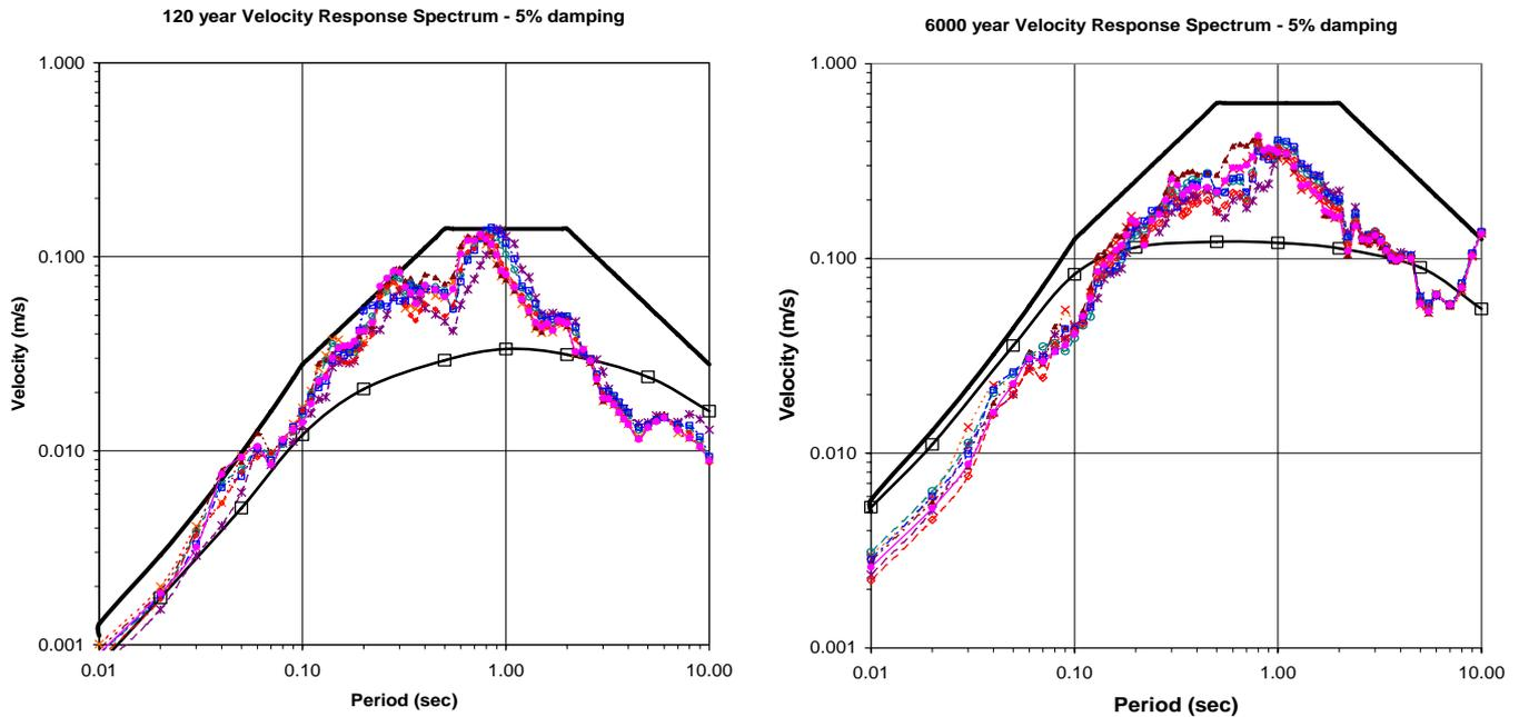
Figure 5 Calculated bedrock and soil surface response spectra
