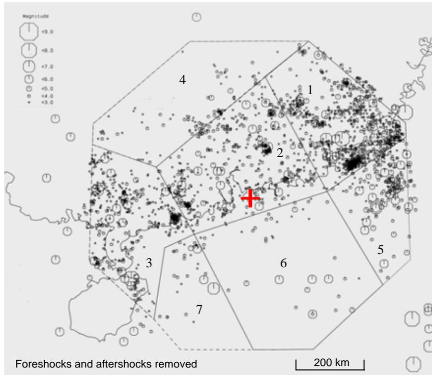
Figure 3 Seismic source model adopted for the seismic hazard assessment
