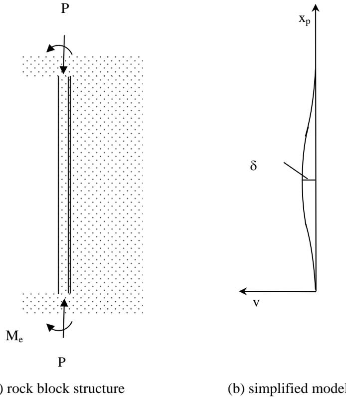
Figure 1 Deformation of rock block structure and analytical model
