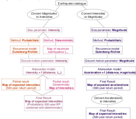
Figure 2. Steps of regional seismic hazard analyses in SISMIMUR approach (in blue) and in SISMICAT and GEOBAL approach (in red/magenta).
