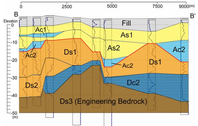
Figure 8 Soil profile along the line No. 5
