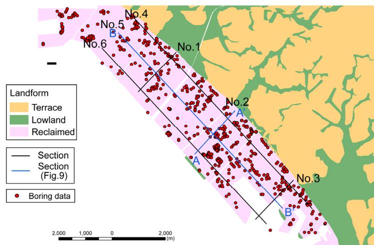
Figure 6 Borehole locations and soil profile lines
