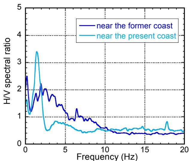
Figure 5 Typical H/V spectra in blocks E and F
