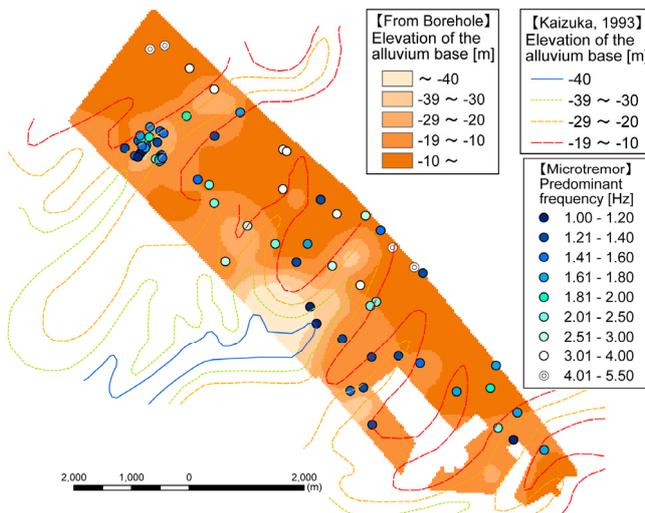
Figure 9 Depth of the alluvium base
