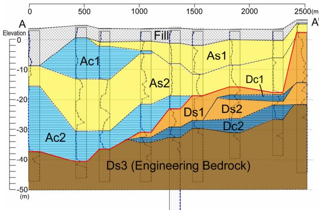
Figure 7 Soil profile along the line No.2
