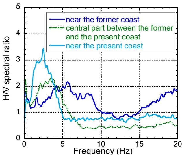
Figure 4 Typical H/V spectra in blocks A, C and D
