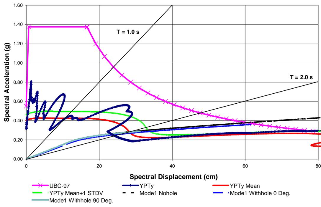
Figure 3 Mode 1 Capacity Curves vs. YPTy Demand Curves
