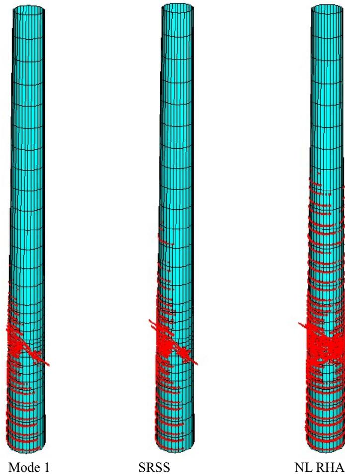
Figure 6 3D Cracking Patterns for Failure of the Model with the Opening
