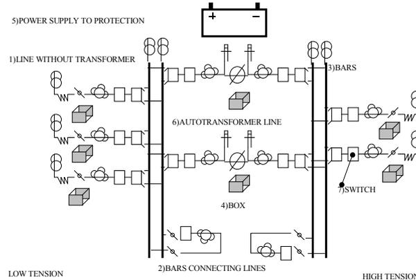
Figure 2. Components in a sub-station.
