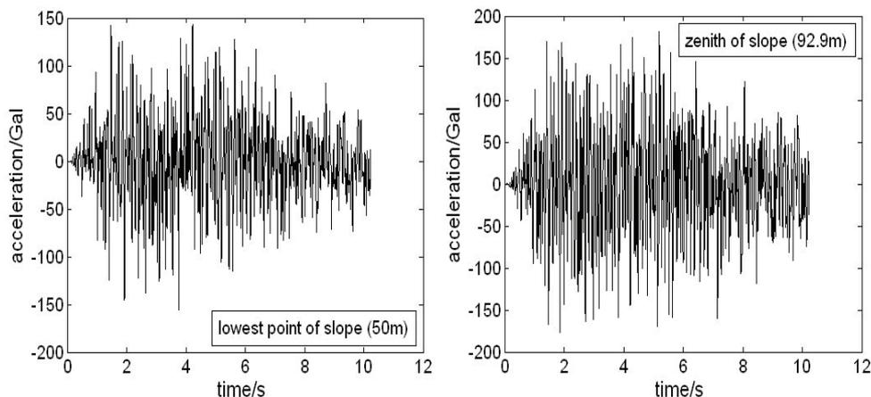
Fig. 5 Seismic response time series in Point-L and Point-Z of slop
