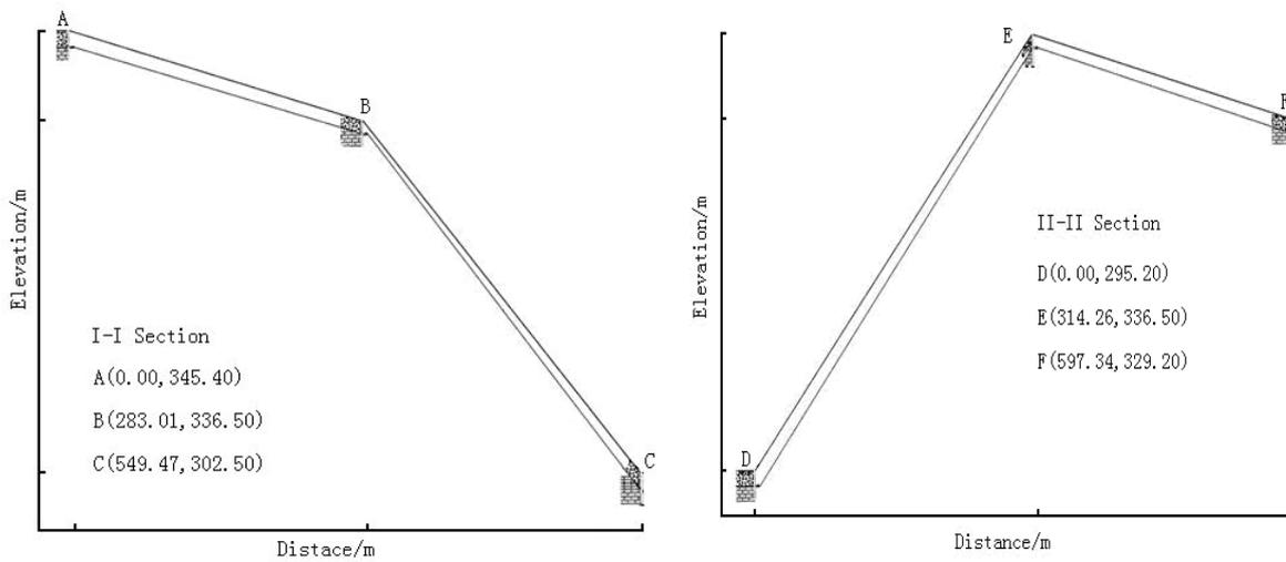
Fig.1 Two slopes of some planned power station
