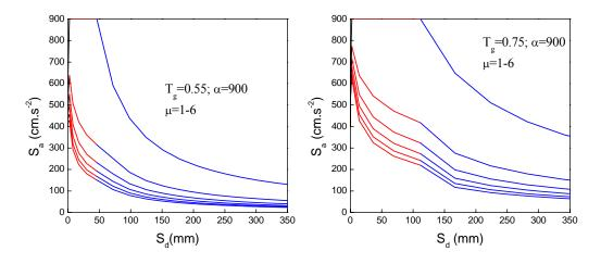
(c) The demand spectra under 8 degree Infrequence Earthquake of III site condition
