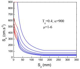
(b) the demand spectra under 8 degree Infrequence Earthquake of II site condition
