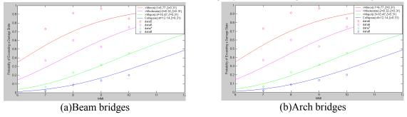
Figure 1: The fragility curve of bridges
