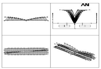
Fig.5 First vibration mode of bridge
