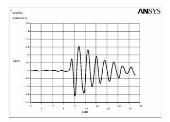
Fig.14 Displacement time history of main wing at tip in lateral direction (unit: m)
