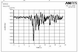
Fig.11 Maximum stress time history of main girder at center of span
