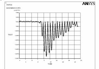
Fig.13 Maximum stress time history of main girder at its bottom(unit: Pa)
