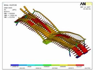
Fig.7 Bridge displacement along bridge axis
