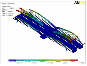
Fig.8 Bridge displacement across bridge axis
