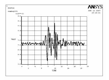
Fig.12 Displacement time history of main wing at tip in longitudinal direction (unit: m)
