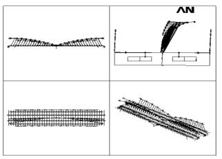
Fig.6 Second vibration mode of bridge
