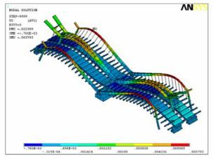
Fig.9 Displacement response in vertical direction
