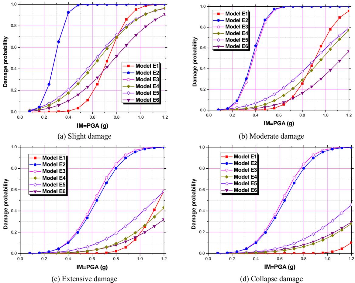
Figure 2 Fragility curves of six bridge models under seismic shaking
