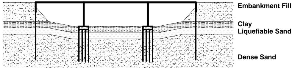
Figure 3 Sketch of simulation for bridge and soil profile with liquefiable sand layer
