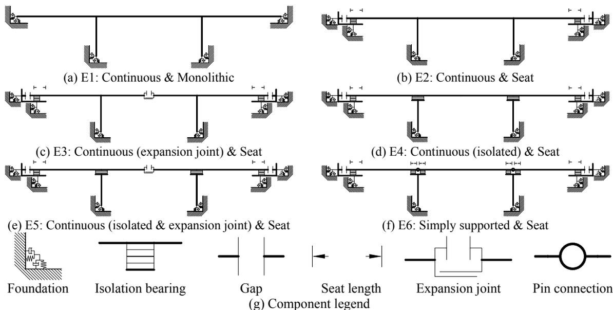
Figure 1 Sketch of six types of bridges
