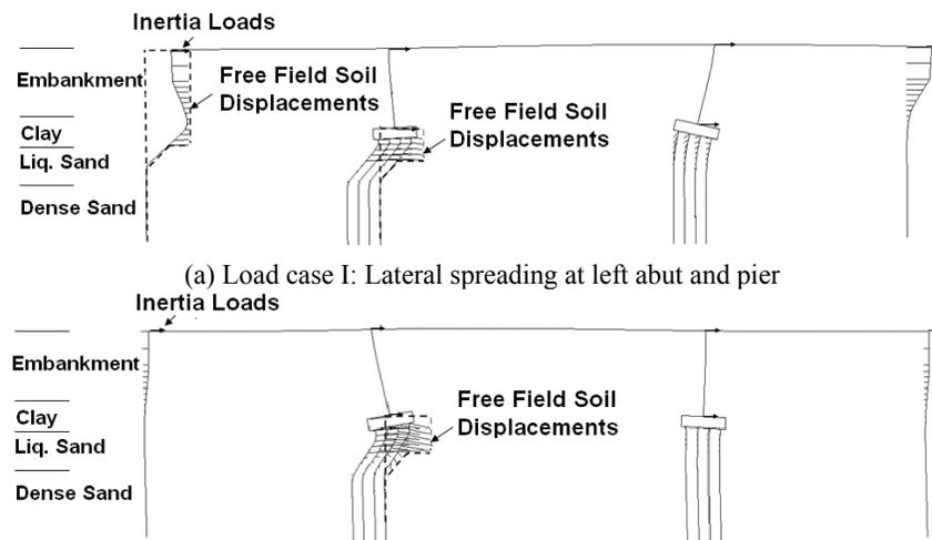
(a) Load case I: Lateral spreading at left abut and pier
