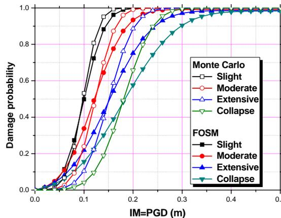
Figure 5 Fragility curves generated with Monte Carlo method or FOSM
