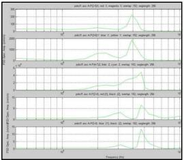
Figure 5. Power Spectral density of signals measured at Villabonita bridge. The upper graps correspond to x,y and z component and bottom graphs represent transfer function in x and y component.
