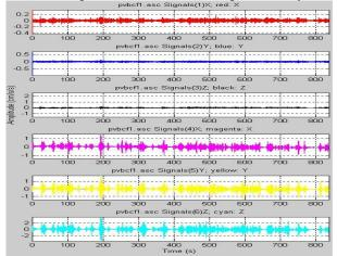
Figure 4 Accelerations measured in two sensors with 3 channels (x = longitudinal, y = transversal and z = vertical) in up to down order. Upper signals belong to free field and the bottom ones to deck of Villabonita bridge.
