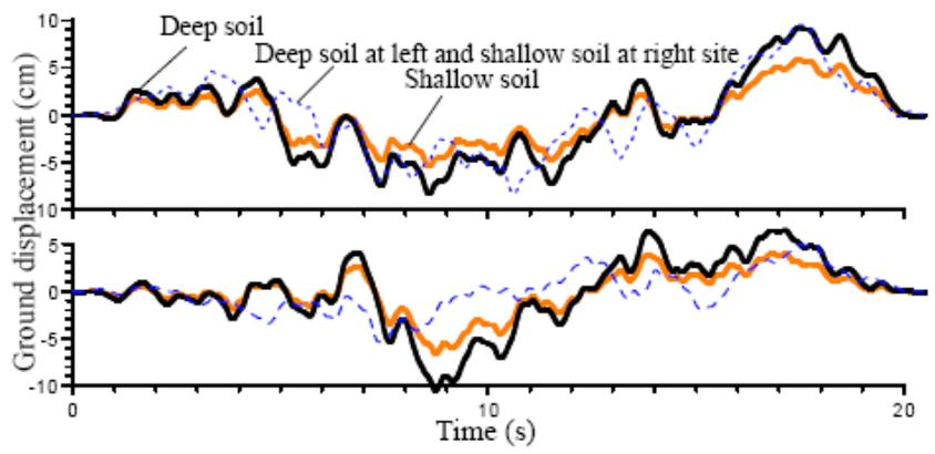
Figure 3. Influence of site amplification on the development of ground displacements at local sites
