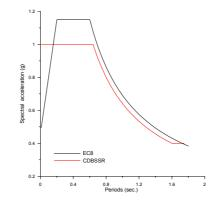
Figure 2 Comparison of spectra acc. EC8 and CDBSSR
