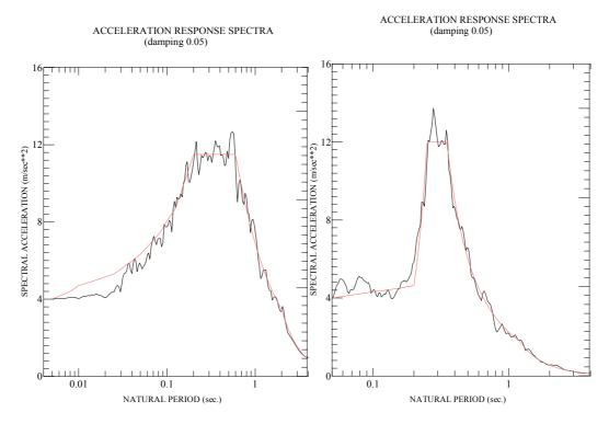
Figure 11. Horizontal and vertical direction - comparison between generated and target response spectra
