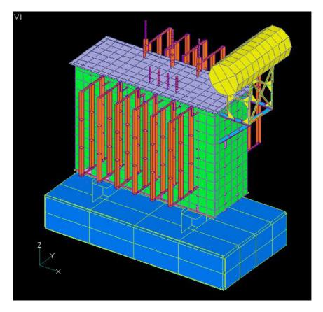
Figure 6 The complex FE model - transformer and foundation
