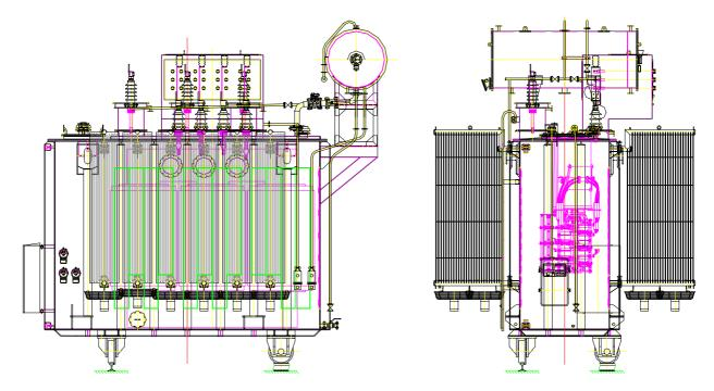
Figure 1 General drawing of the transformer
