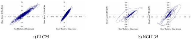
Figure 7 Structure hysteresis curves for selected record
