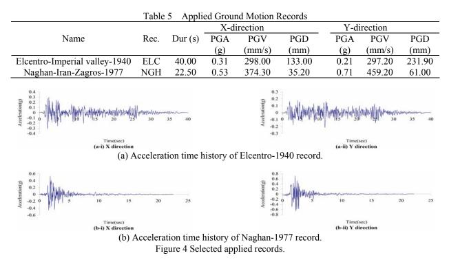
In order to evaluate the behavior of the system under different level of shaking the dynamic loading applied on the specimen in both E–W and N–S directions simultaneously by two level of excitation, respectively low-level and high level seismic excitations. The description of shaking levels is presented in Table 6.
