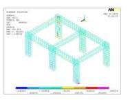
c) Tensile stress in steel mesh of panels d) Tensile stress in reinforcement Figure 10 Stress distribution under NGH135 record at 1.155 s (inkN/mm2)
