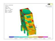
a) Tensile stress in concrete
