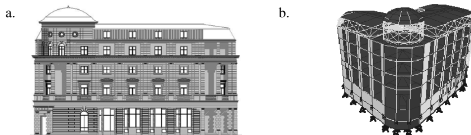
Figure 7 View of 6-story base isolated commercial center-hotel of “Tufenkian Hospitality” LLC on Hanrapetutyán Street in Yerevan (a) and its design model (b)
