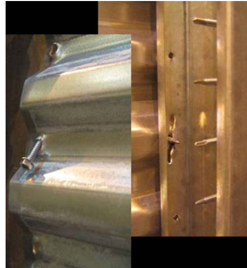
Figure 4. Typical CSSSW Group Response and Failure Mode
