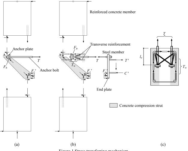
Figure 1 Stress transferring mechanism
