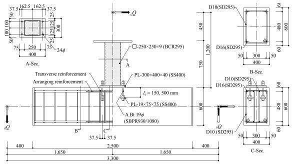
Figure 2 Details of test specimens
