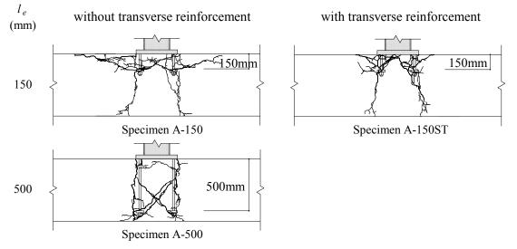
Figure 4 Crack Patterns
