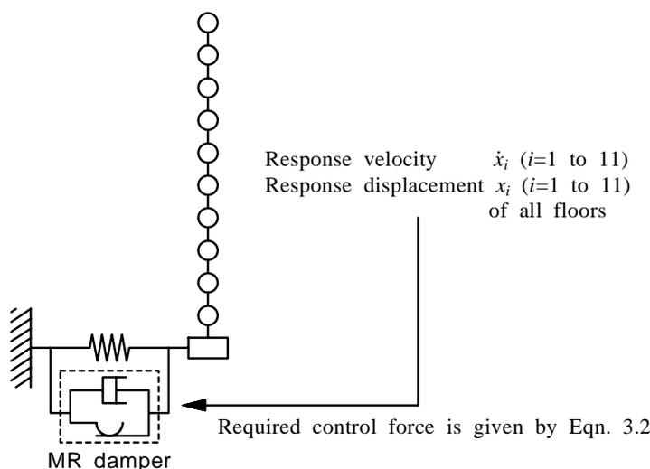
Figure 3. Optimal control by linear quadratic regulator theory
