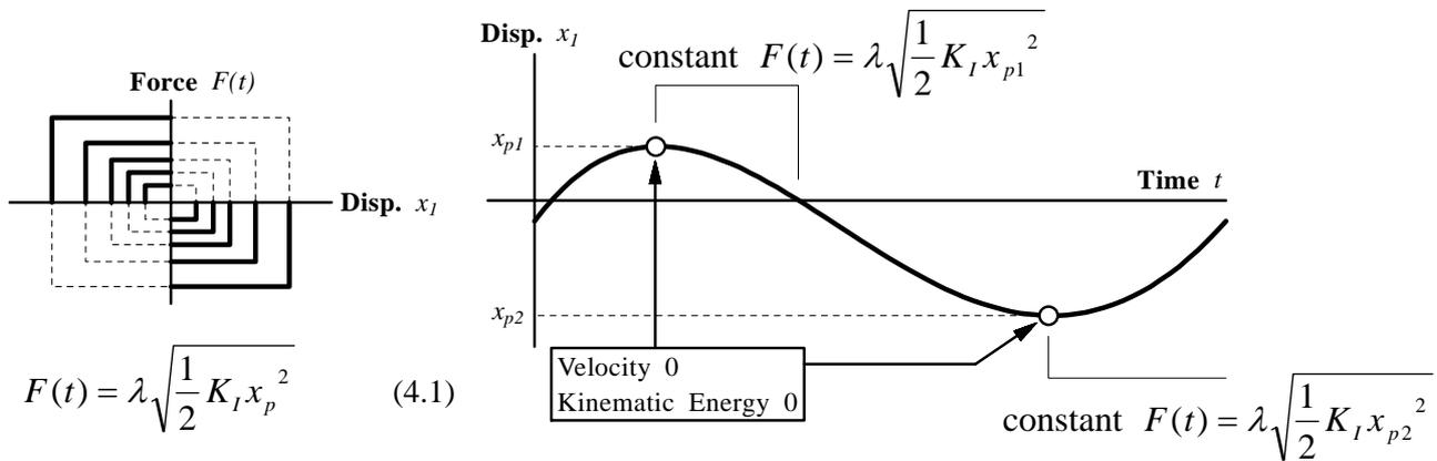
Figure 6. Determination of control force in the second and fourth quadrant
