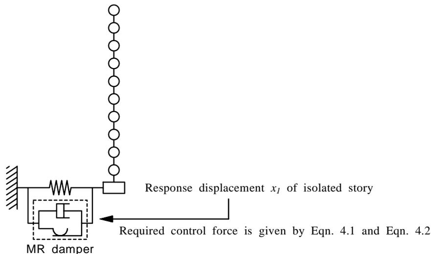
Figure 8. Proposed control by response displacement of isolated story
