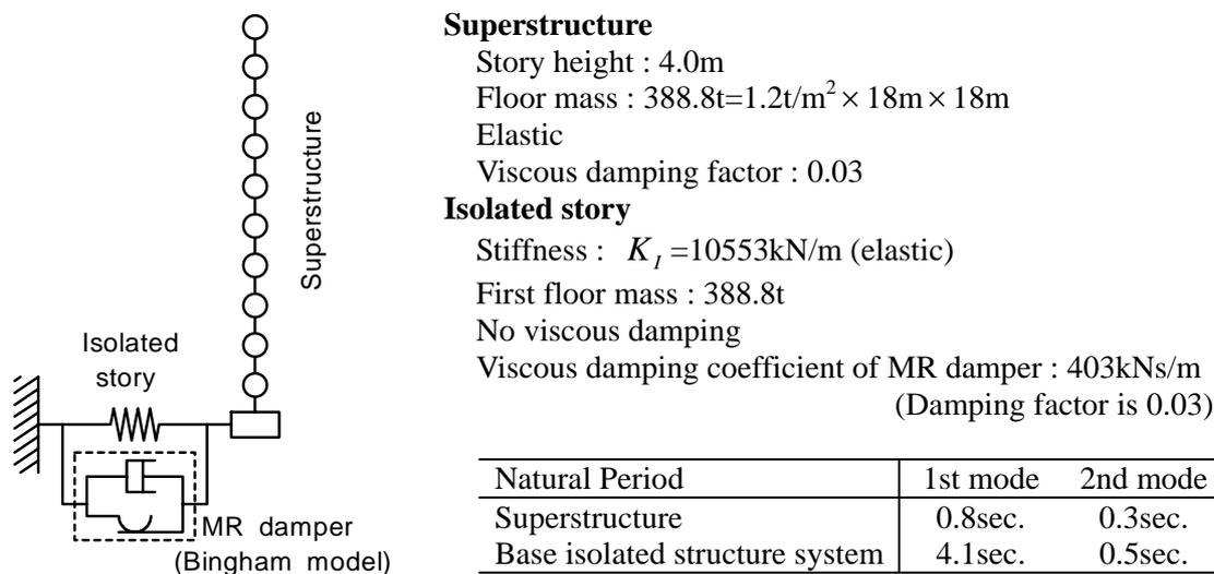
Figure 1. Analytical model of subjected base isolated structure
