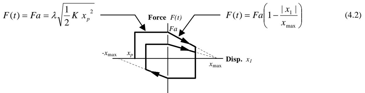
Figure 7. Control force of proposed control method
