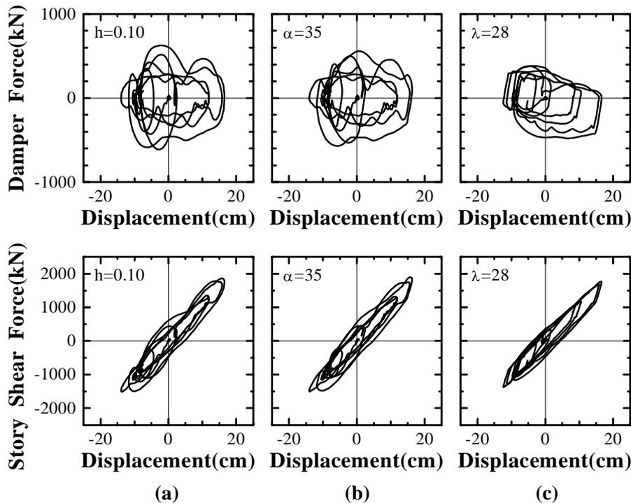
Figure 10. Hysteresis loop of damper and isolated story with various dampers (JMA Kobe NS):
