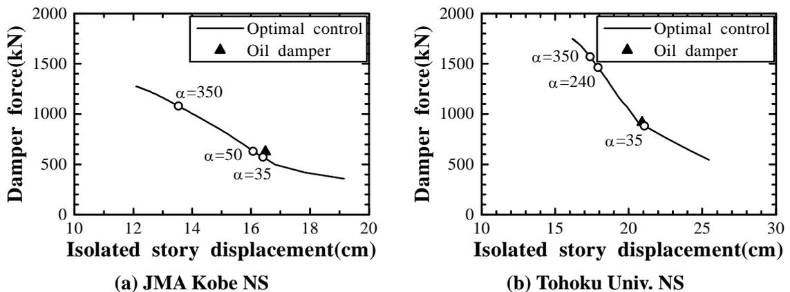
Figure 5. Maximum response values of damper force and isolated story displacement with various  $\alpha$
