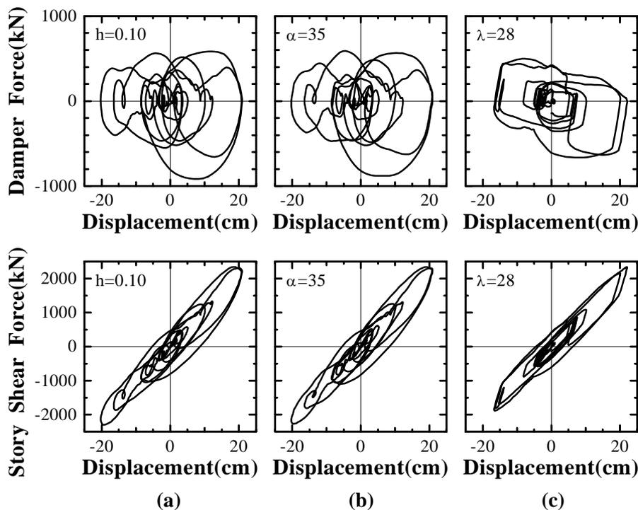
Figure 12. Hysteresis loop of damper and isolated story with various dampers (Tohoku Univ. NS):
