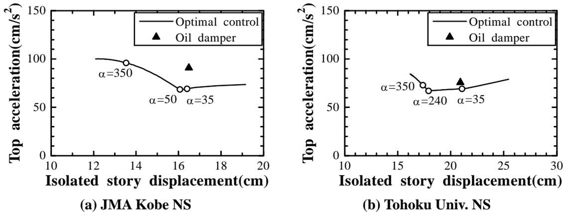
Figure 4. Maximum response values of top acceleration and isolated story displacement with various  $\alpha$
