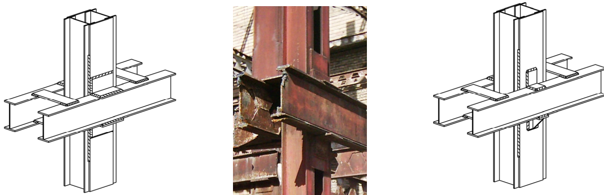
Figure 1: Two common details of typical Iranian Khorjini connections [4, Photo: B.Shafei]
