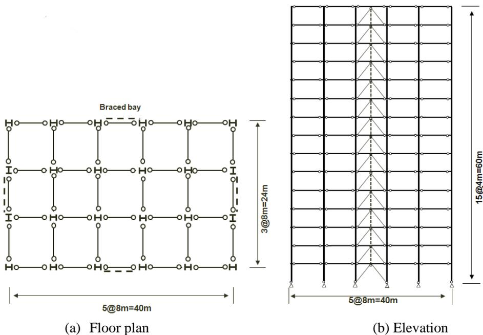
Figure 5 Floor plan and elevation
