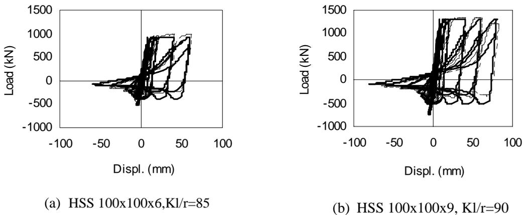
Figure 4 Comparison of experimental and numerical results (---: experimental, — : numerical)
