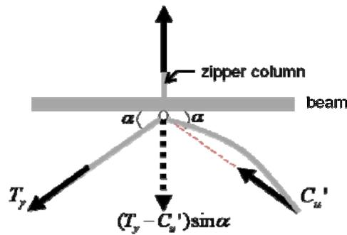
Figure 3 Postbuckling vertical unbalance force
