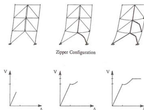
Figure 1 Improved performance by zipper column configuration (Khatib et al 1988)
