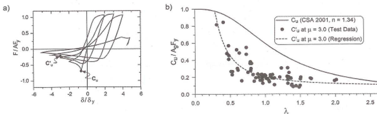
Figure 2 Cyclic behavior of bracing members and residual postbuckling strength [Tremblay, 2002]
