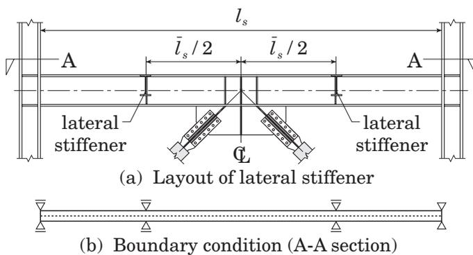
Figure 7 Boundary condition of girder
