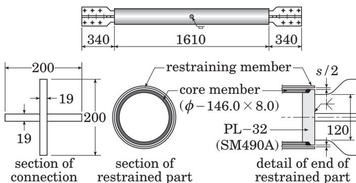
Figure 10 Detail of buckling-restrained brace
