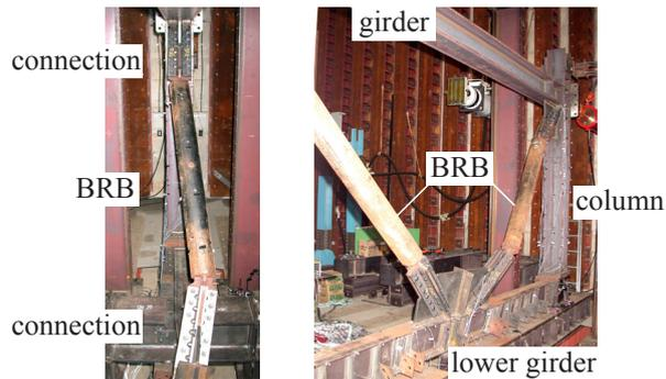
Photo 1 Specimen after occurring out-of-plane buckling
