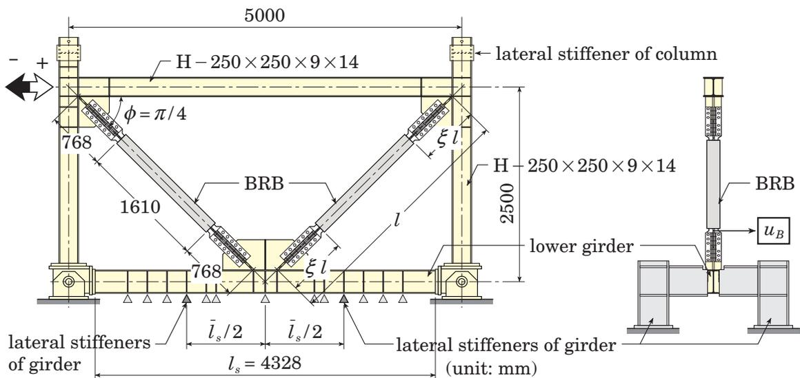
Figure 9 Test setup
