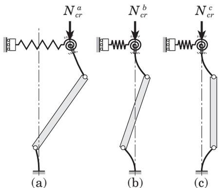
Figure 4 Out-of-plane buckling mode
