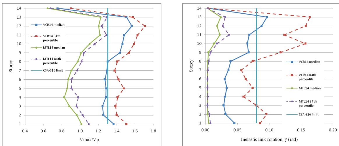
Figure 3.1 14-storey frame: Normalized maximum link shear forces and deformations
