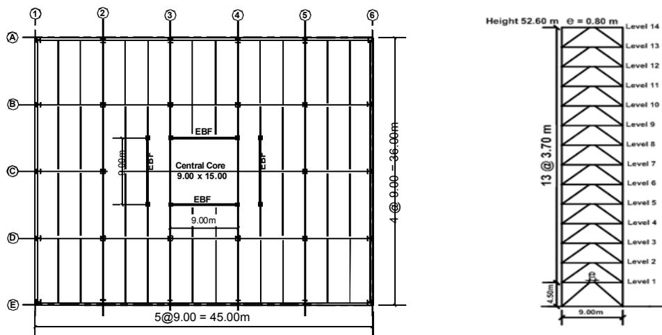
Fig.2.1. Layout and the elevation of the fourteen-storey EBF
