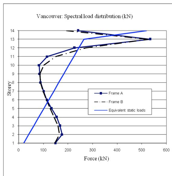
Fig. 2.2 Lateral force distributions obtained from the spectral analysis
