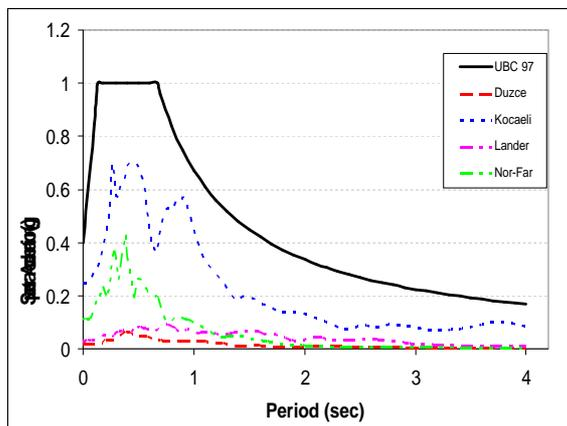
Figure 3: Far-Field earthquake acceleration spectra
