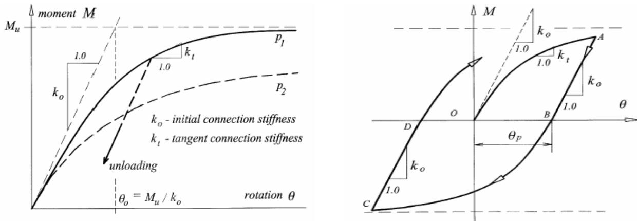
Figure1: a) Three-parameter power model, b) Independent hardening model
