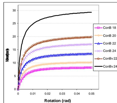
Figure 2: moment-rotation curve for TSAW connections
