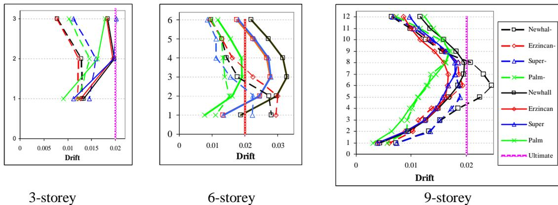
Figure 5: Comparison between the drifts of 3, 6 and 12-storey rigid and semi-rigid frames under near-field earthquake records
