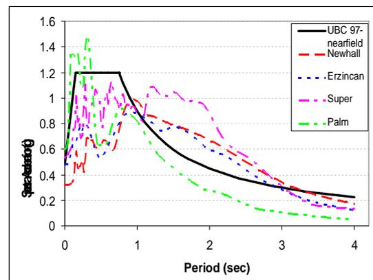
Figure 4: Near-Field earthquake acceleration spectra
