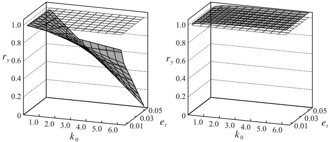
(a) The case that connection yield precedes beam yield (Frame A)      (b) The case that beam yield precedes connection yield (Frame A)
