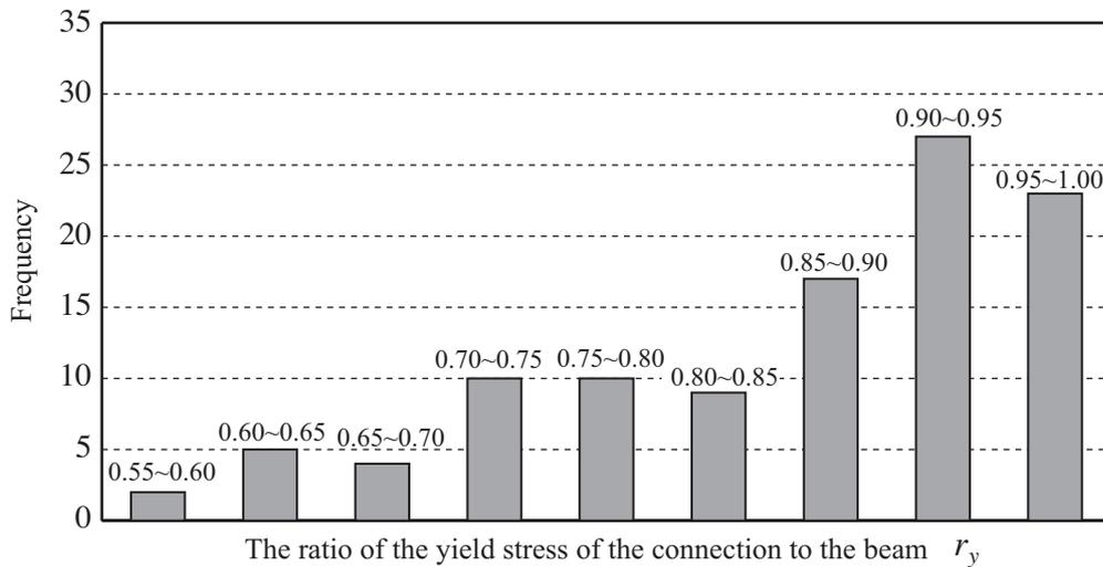
Figure 7 Frequency distribution of yield-limited ratio for the designed connection
