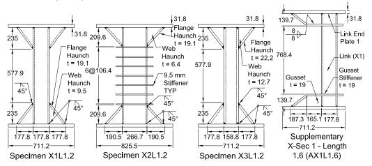
Figure 3. Example Link Specimen Elevations
