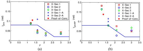
Figure 4. Limit Plastic Rotation versus Normalized Link Length (a) Experimental Results (b) Projected for 2005 Loading Protocol
