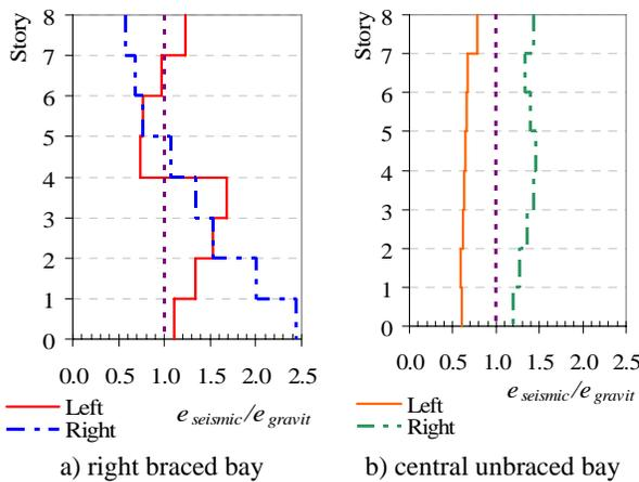
Figure 12. Beams stress ratio of the central bay, Ch8p6 model
