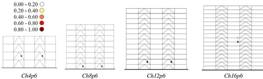
Figure 7. Initial yielding for models where columns resist near 65% of the total seismic shear force.
