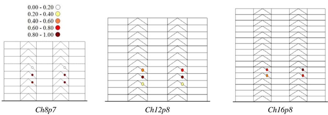
Figure 9. Initial yielding for models where columns resist near 75% of the total seismic shear force.
