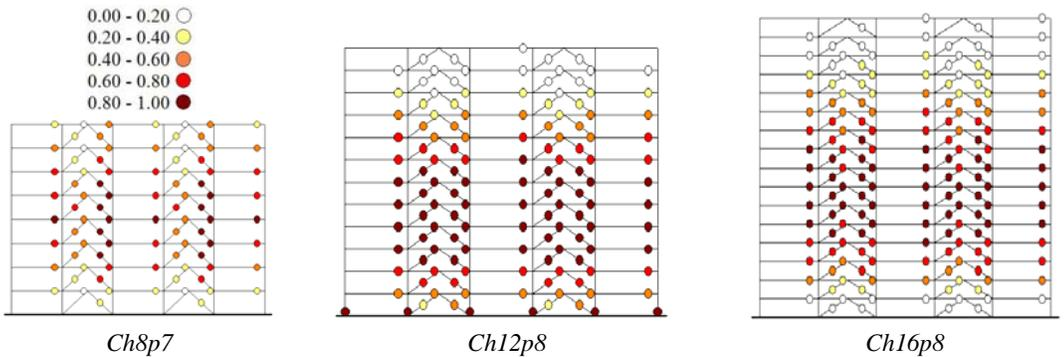
Figure 10. Final collapse mechanisms for models where columns resist near 65% of the total seismic shear force
