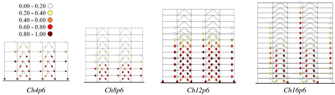
Figure 8. Final collapse mechanisms for models where columns resist near 65% of the total seismic shear force
