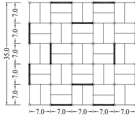
Figure 2. Floor plan of the building in meters
