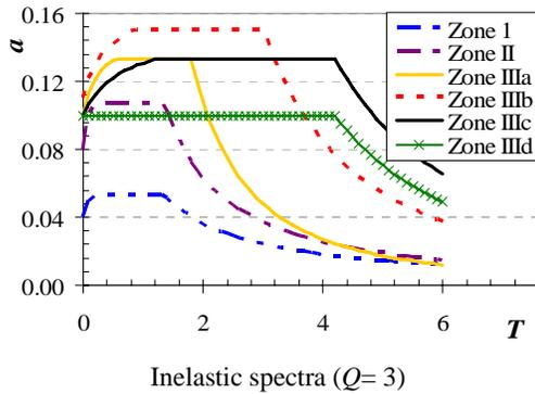
Figure 1. Design spectra according with MFDC-04
