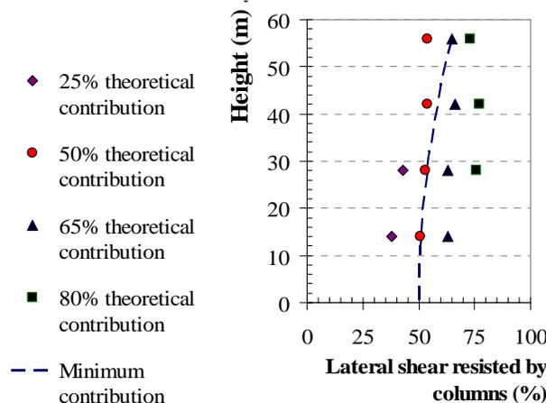
Figure 11. Minimum percentage of seismic shear force resisted by the columns.
