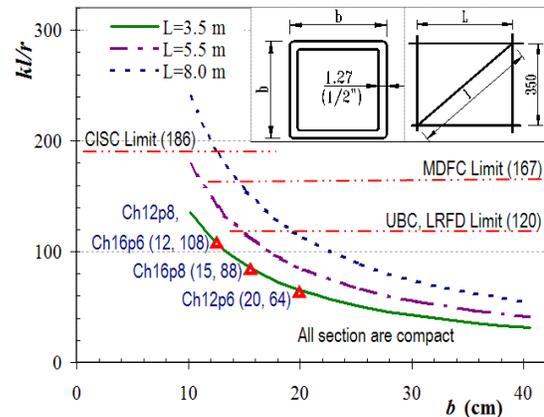
Figure 16. Review of slenderness ratio and compact section criteria for the braces of box section used.
