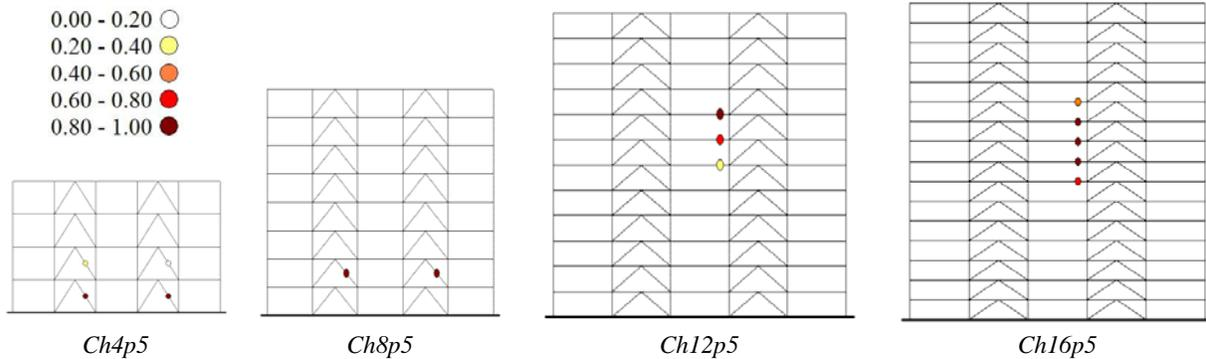
Figure 5. Initial yielding for models where columns resist near 50% of the total seismic shear force
