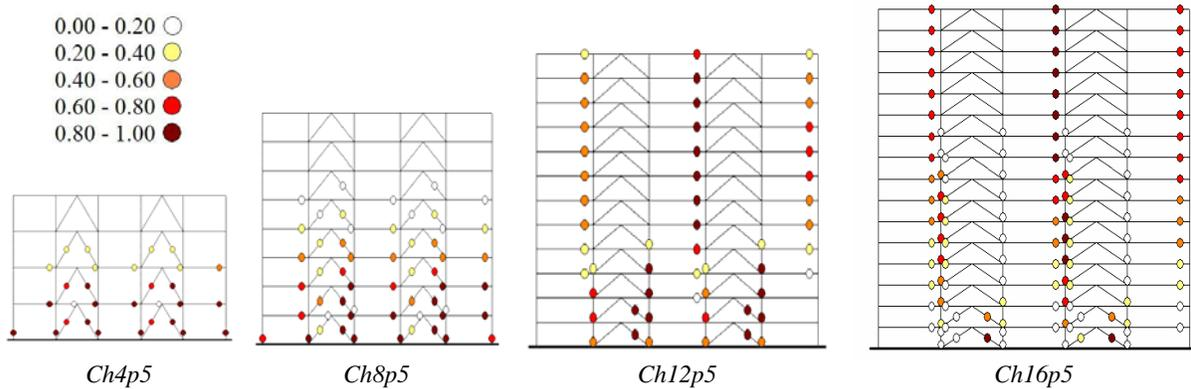
Figure 6. Final collapse mechanisms for models where columns resist near 50% of the total seismic shear force
