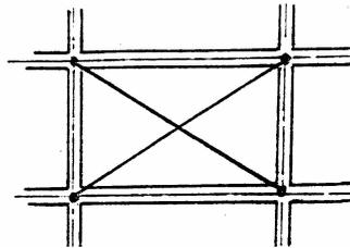
Fig 6 Idealisation of infill for dynamic analysis
