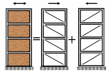
Fig 7 Idealisation of in filled frame building
