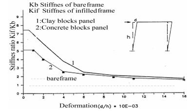
Figure 2 Degradation of panel stiffness
