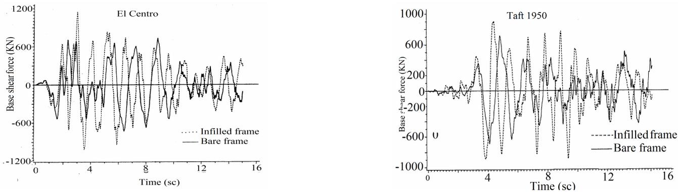
Fig 13 Effect of infill panels on the seismic base shear force
