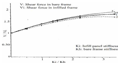
Fig 12 Effect of infill panels on the seismic base shear force
