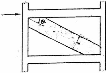
Fig 5 Idealisation of masonry Infill panel
