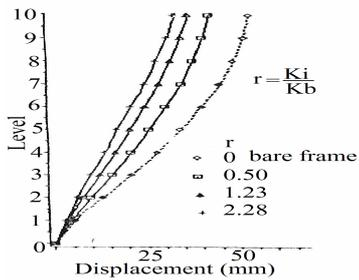
Fig 14 Maximum floor displacements (Taft earthquake)
