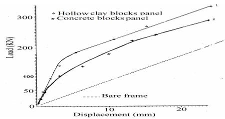
Fig. 3 Experimental strength envelop vs displacement curves
