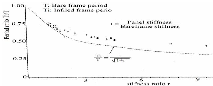
Fig 11 Effect of infill panel on the fundamental period
