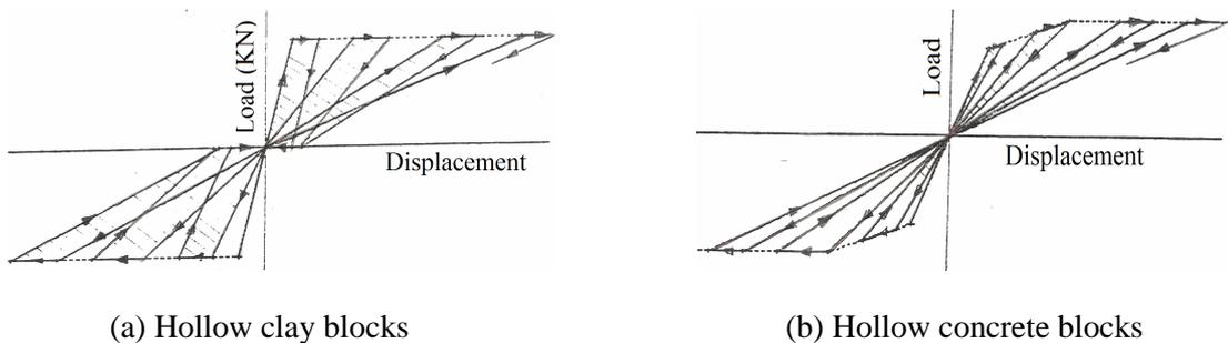
Figure 4: Hysteretic model of infill panel
