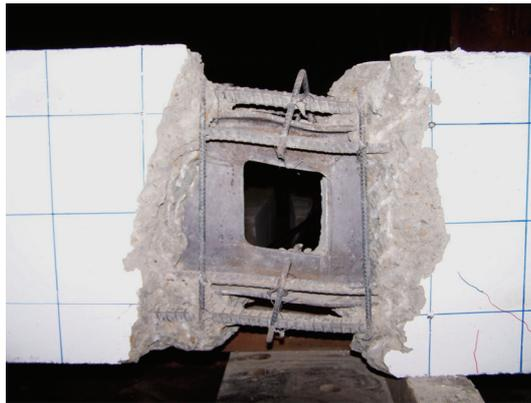
Figure 6 Shear deformation of the steel web of specimen S4
