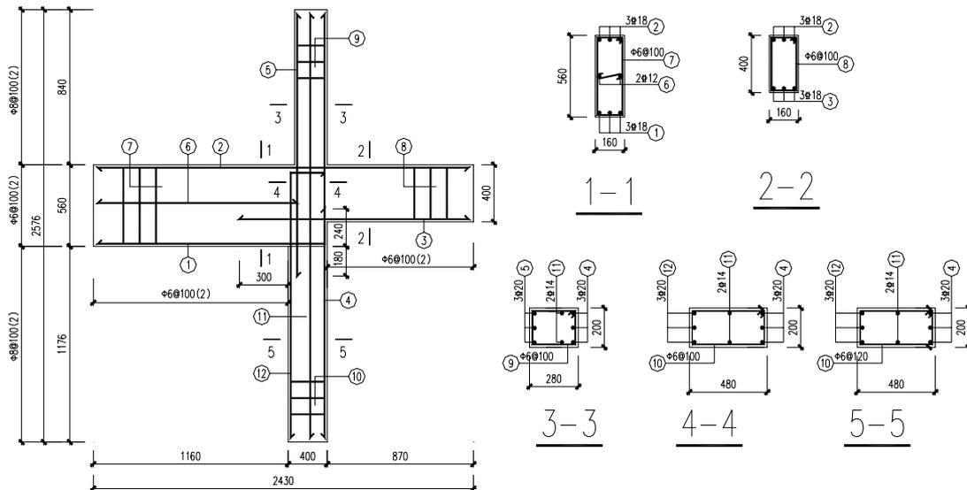
Figure1 Dimension and steel arrangement of J-2
