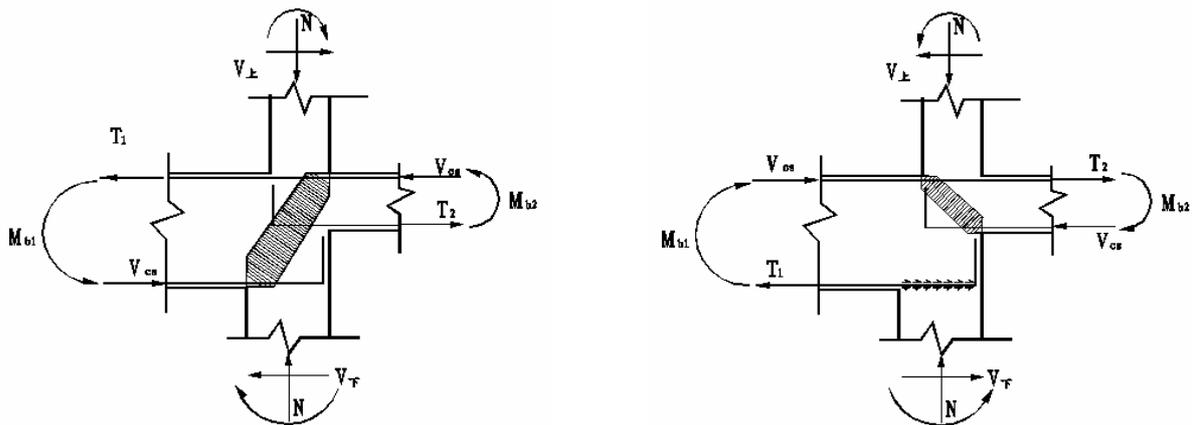
(a) Big beam bearing the positive bend moment (b) Big beam bearing the negative bent moment
