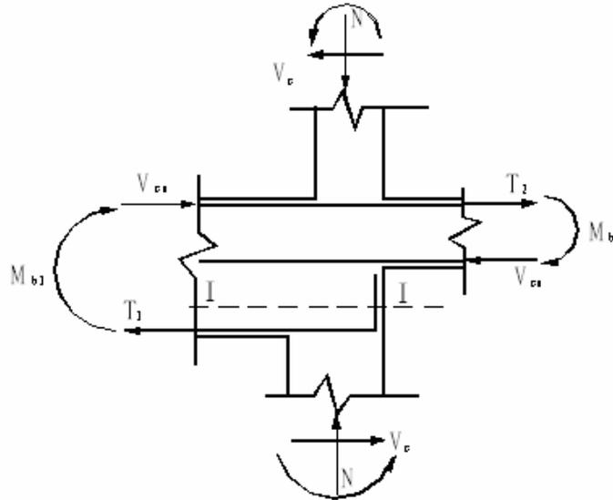
Figure 7 Mechanism of the column shear failure
