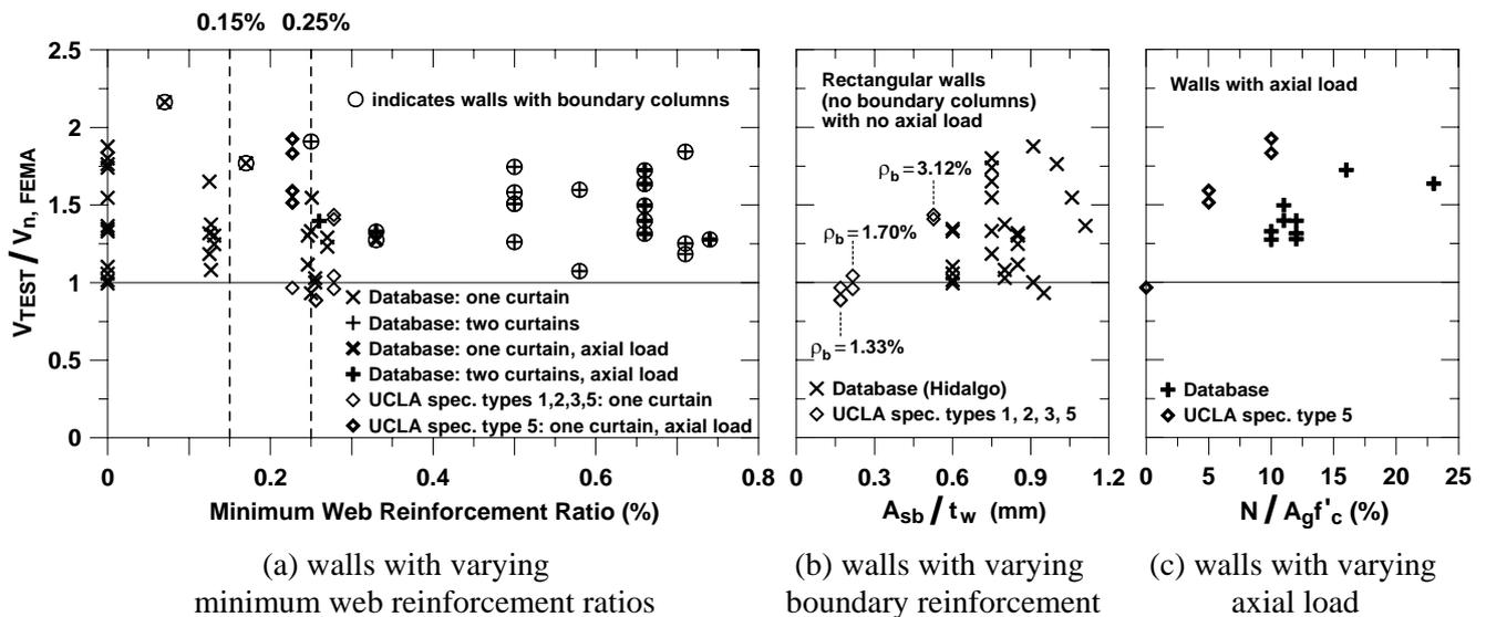
Figure 3 Comparison of wall test data with FEMA 356 nominal shear strength calculation.
