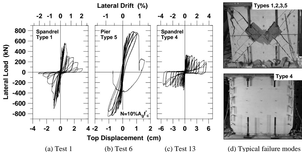
Figure 2 Representative lateral load-displacement responses and failure modes for the wall specimens.
