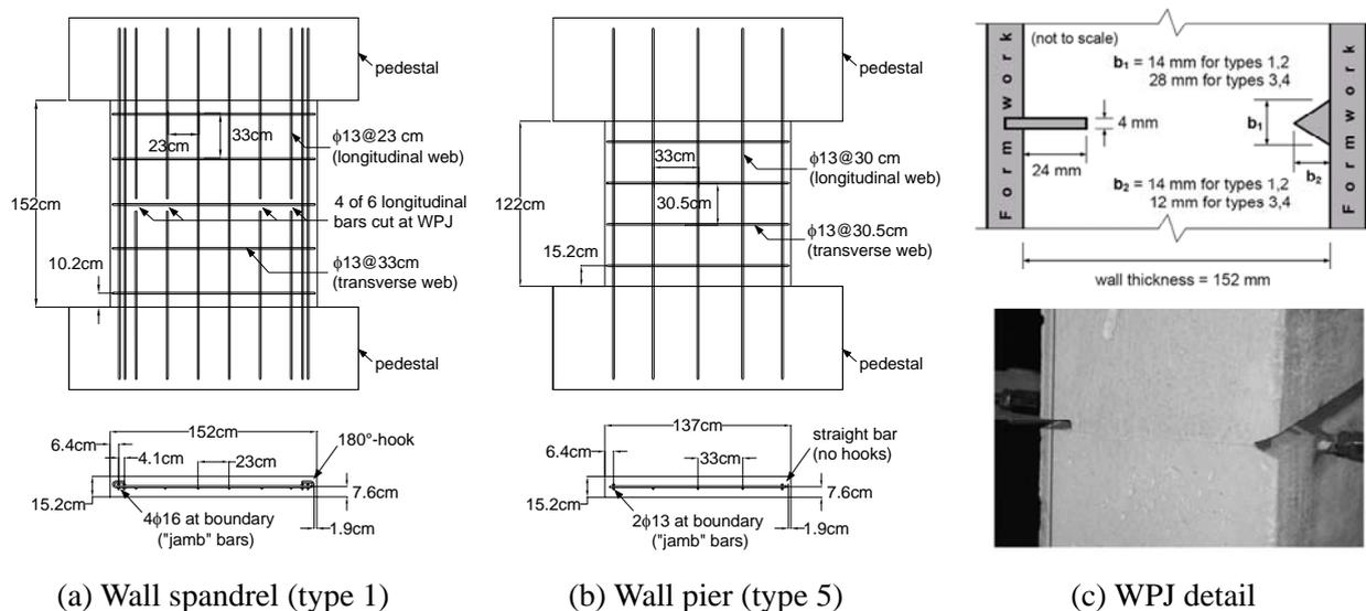
Figure 1 Sample wall specimen geometry and reinforcement.
