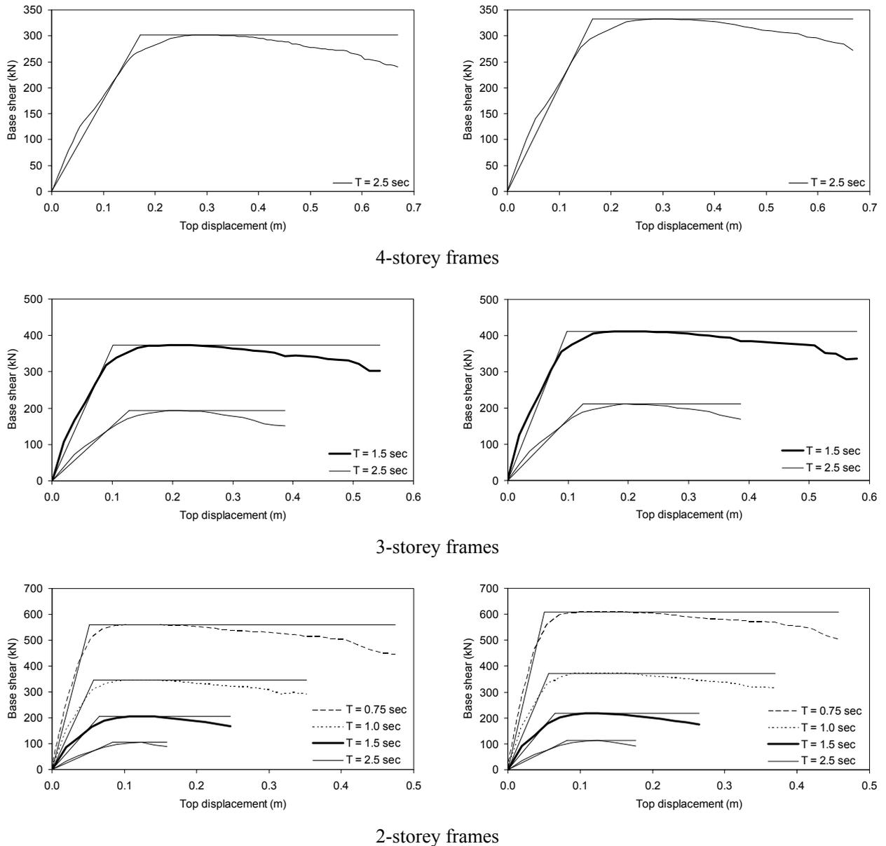
Figure 2. Capacity curves for frames with constant (left) and variable (right) column stiffness.
