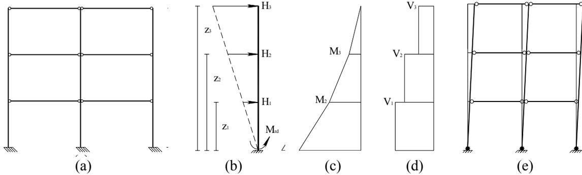
Figure 1. (a) Multi-storey frame with hinged beams, (b) distribution of storey forces, (c) bending moments, (d) shear forces, and (e) desired collapse mechanism.
