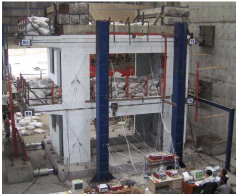
Figure 1 PC-wall panel with precast/prestressed half slab full-scale model and hysteresis diagram
