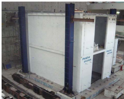
Figure 3 Concrete wall panel with hollow-core slab full-scale model and hysteresis diagram
