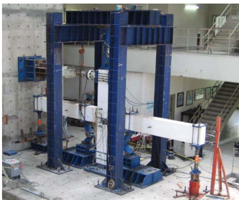
Figure 2 Interior PC-beam column joint full-scale model and hysteresis diagram
